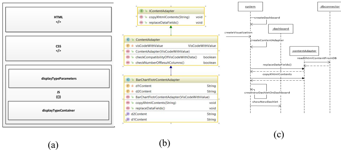
Figure 35 - a) XHTML content for a JavaScript-based display b) ContentAdapter structure for Flotr JavaScript library based Bar Chart visualization c) Sequence diagram for visualization display in dashboard form
