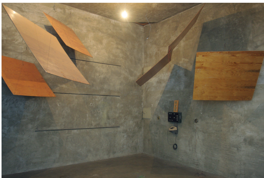
Figure 2.10: A Reverberation Chamber.
