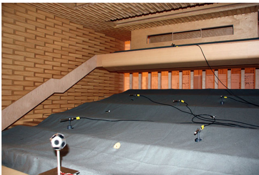
Figure 2.6: Scale model of a chamber music hall.
