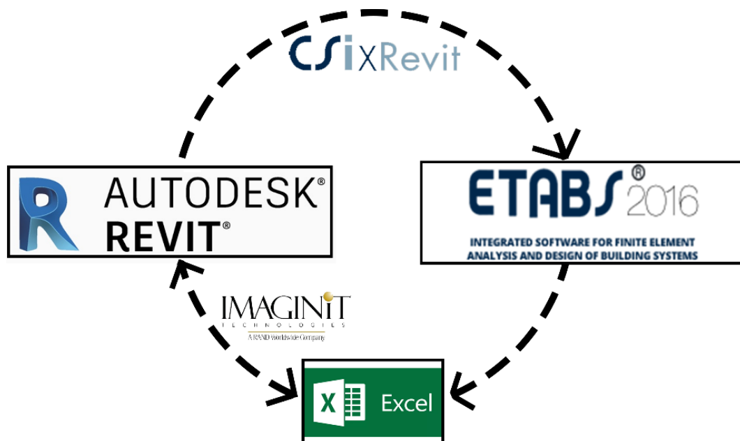
Figure 3.18. Data flow schema used among BIM compatible tools and add-ins
