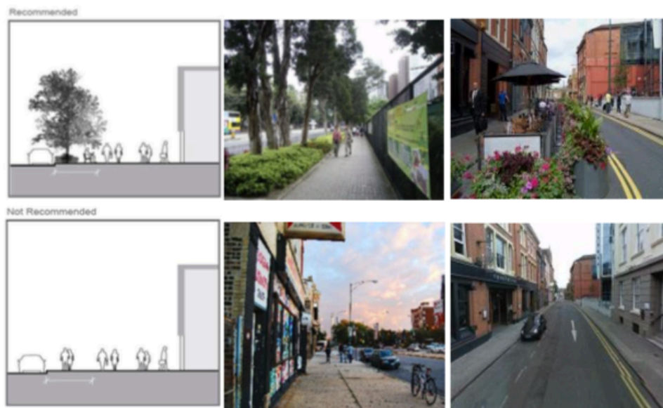
Figure 3.14. Street furniture in walkway enclosure (LA-Walkability, 2008)
