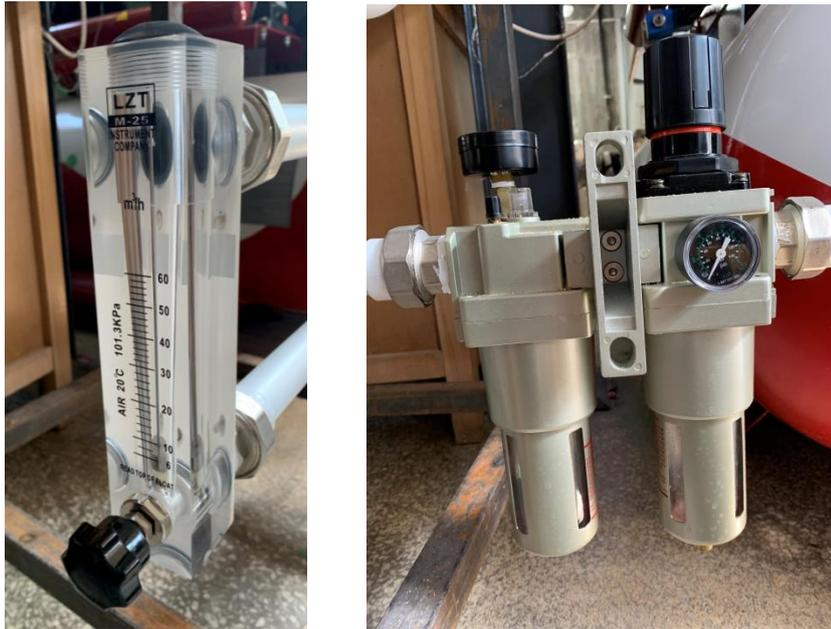
Figure 2.6 Rotameter and pressure regulator
