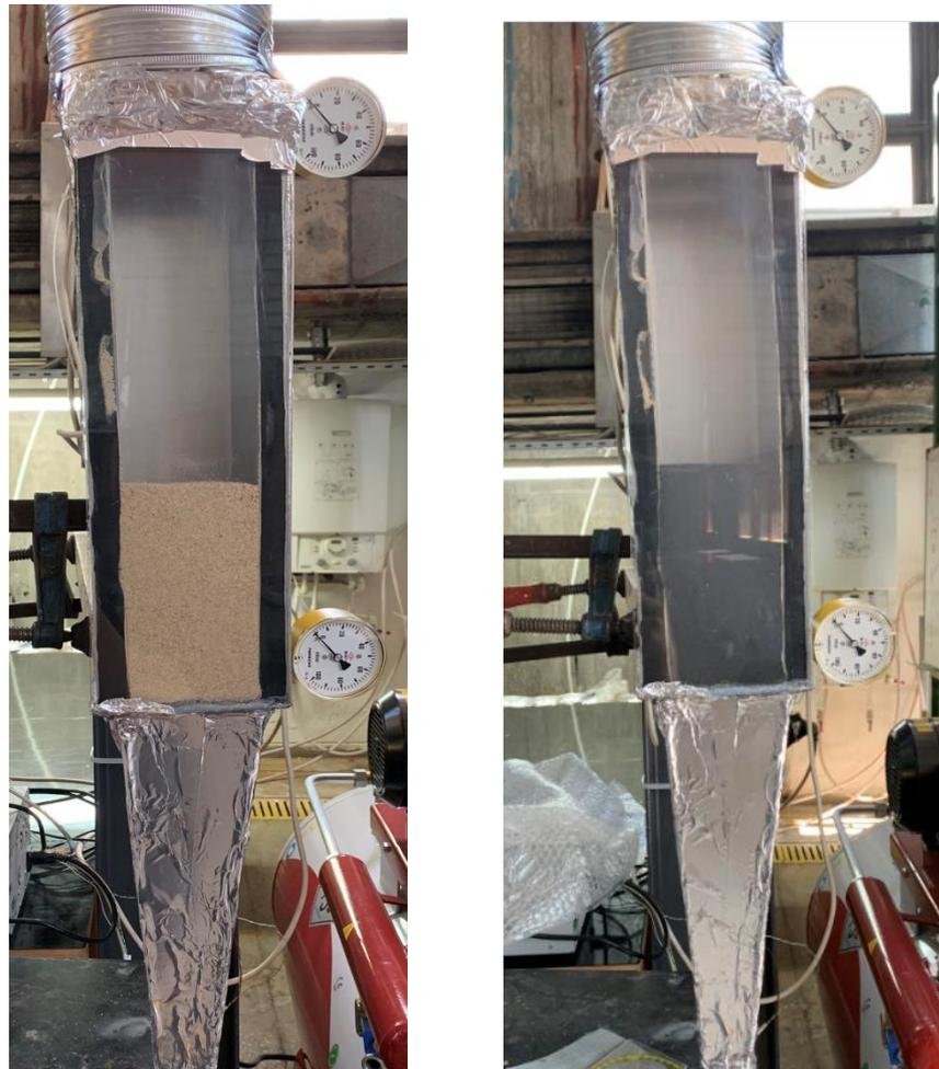
Figure 2.4 Real view of bed with sand and CARBOHSP particles
