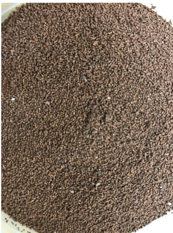
Figure 2.1. Granulated spheres of immobilized glucose isomerase
