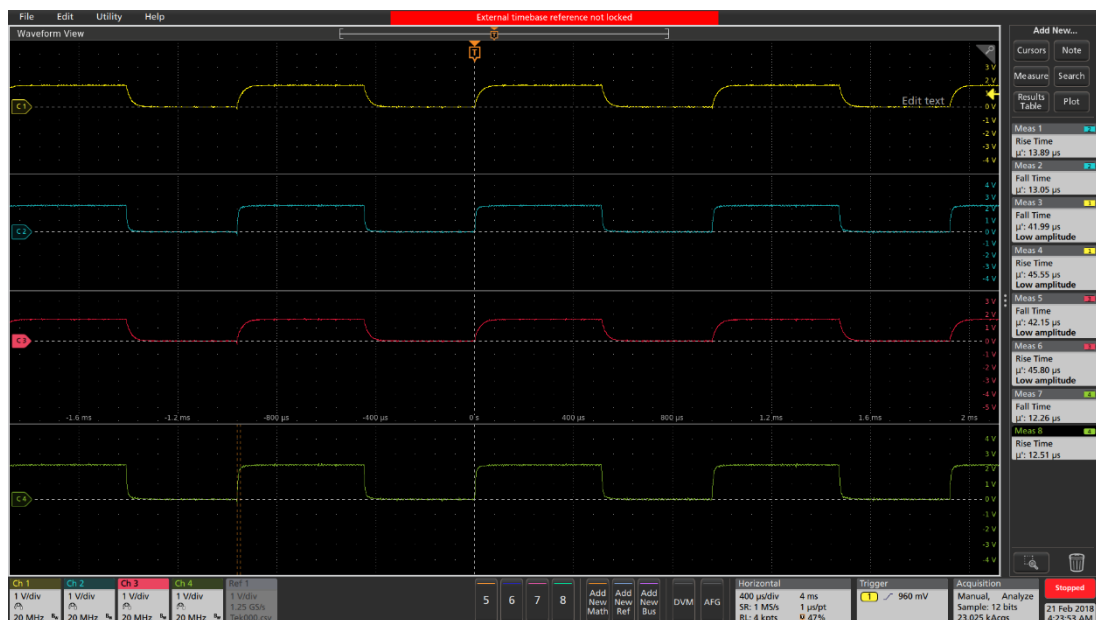
Figure 3.10 Signals transferred from irradiation room to control room before irradiation: Yellow: Sensed-Ids1, Blue: Sensed-Vgs1, Red: Sensed-Ids2, Green: Sensed-Vgs2
