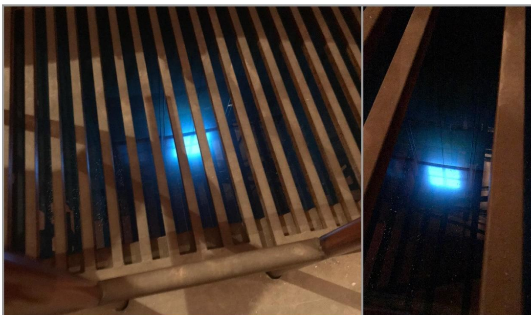
Figure 4.10 Cherenkov radiation when the Co^{60} source is under the water
