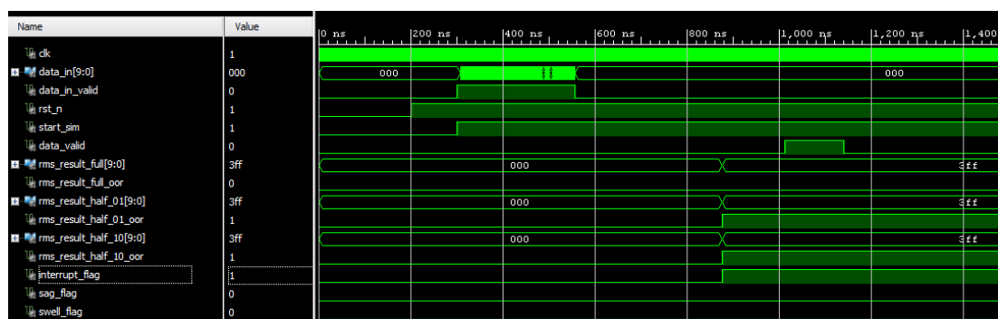
Figure 5.9: Functional Simulation Result with High Interrupt Flag
