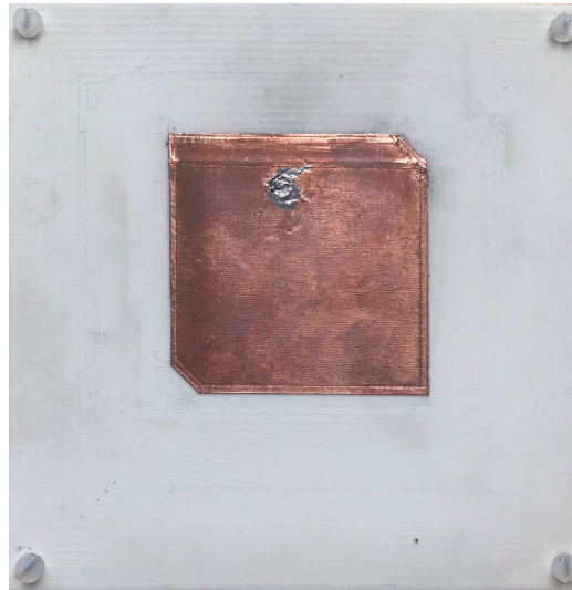
Figure 4.70: Tuned three-layer stacked antenna at L1 GPS band.
