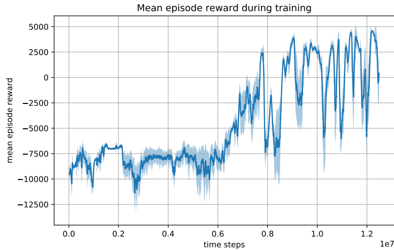
Figure 6.8: Mean episode reward collected during point-to-point training of the bi-rotor without tail. Blue line represents average episode reward in last 200 episodes, and light blue regions are their standard deviation.
