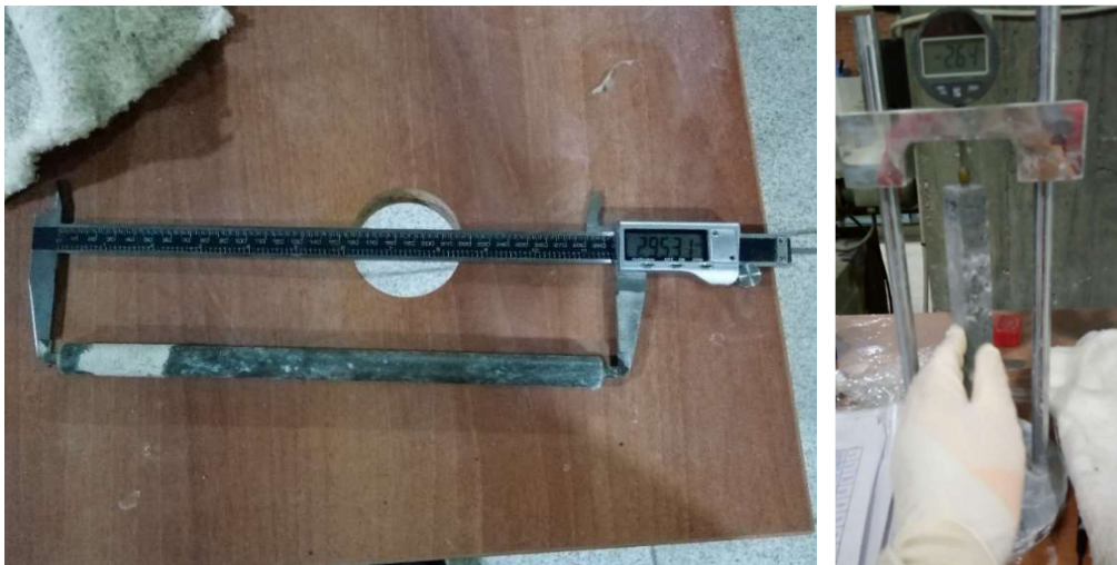
Figure 26. The standard rod used for the comparison of the measurements and the measurement process
