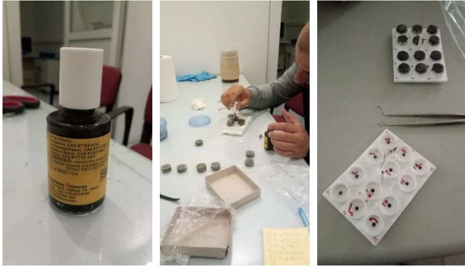
Figure 29. Preparation of the specimens for SEM examination
