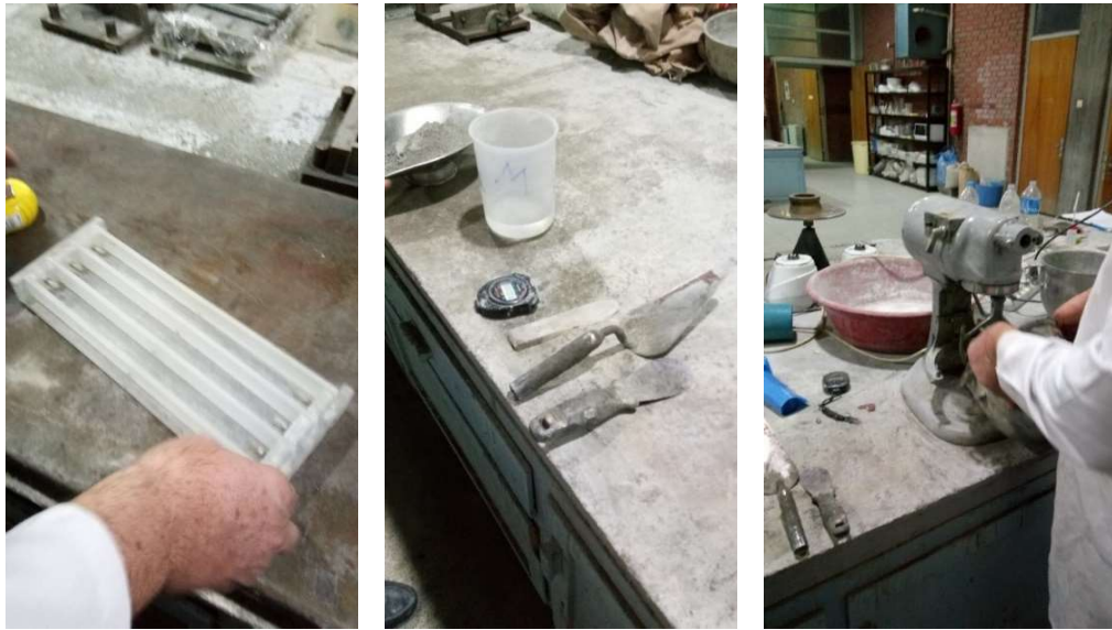
Figure 23 Preparation of the mold, hand tools used and the mixing process
