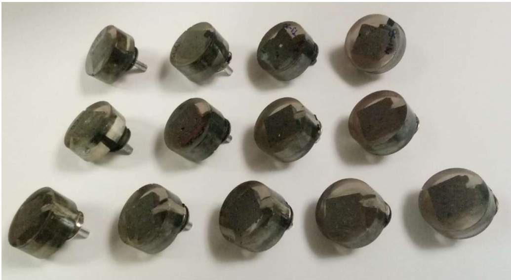
Figure 28. Polished sections prepared for examination through SEM
