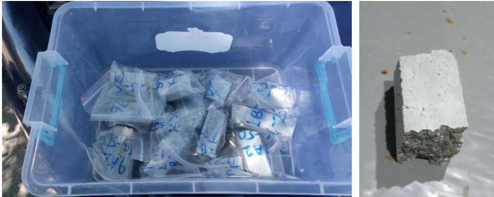
Figure 27. Broken mortar bar specimens for the preparation of the polished sections
