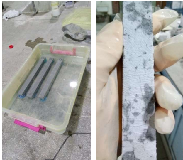
Figure 25. Mortar bars in the NaOH solution and outside
