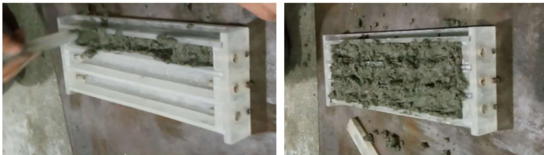
Figure 24. Filling the mold with the fresh mortar
