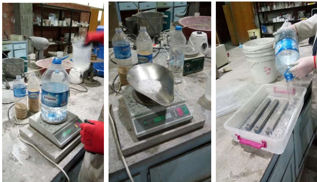
Figure 22. Distilled water, NaOH salt and pouring the mixed solution into the box containing the mortar bars.
