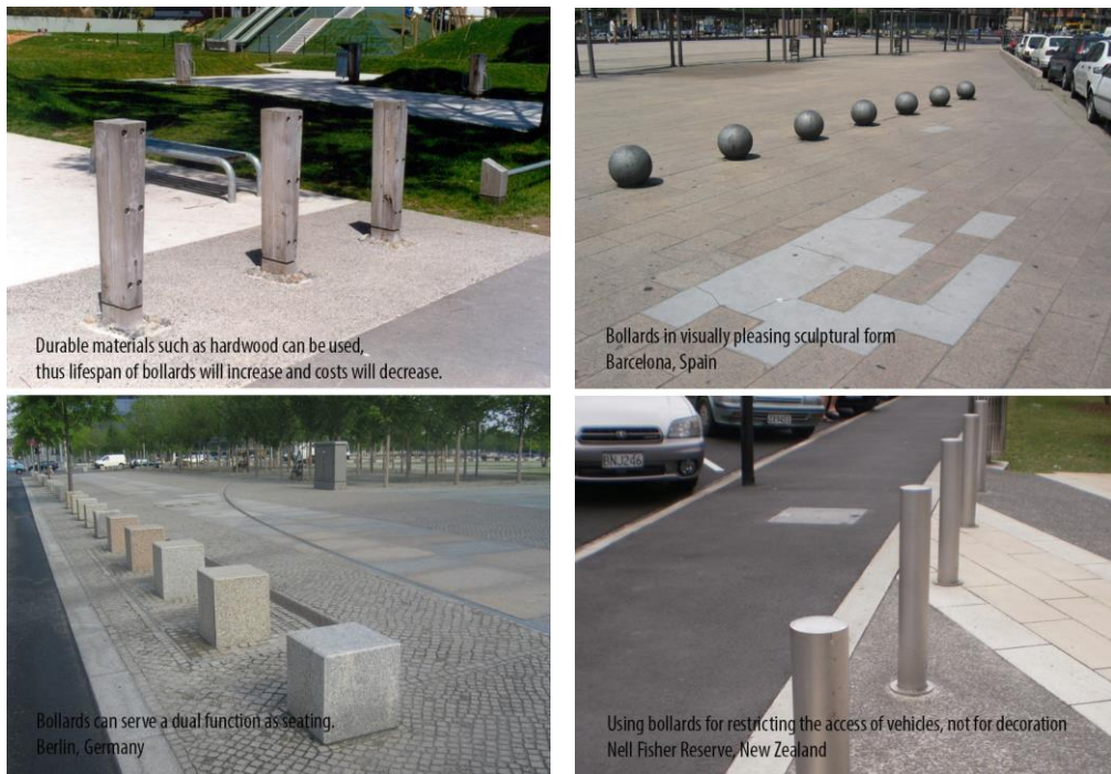
Figure 2-11. Examples of using bollards 22
