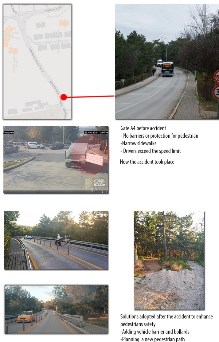
Figure 5-15. Zone 4 (A4 entrance gate) sidewalk width analysis
