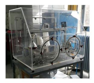
Figure 3.3 Air conditioning glove box
