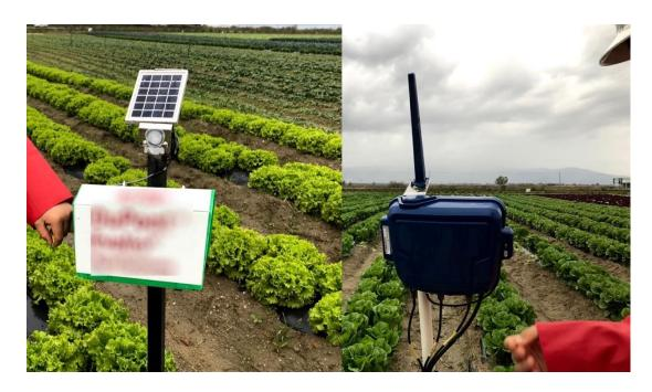
Figure 7.2. Humidity sensor placed inside the lettuce crops.
