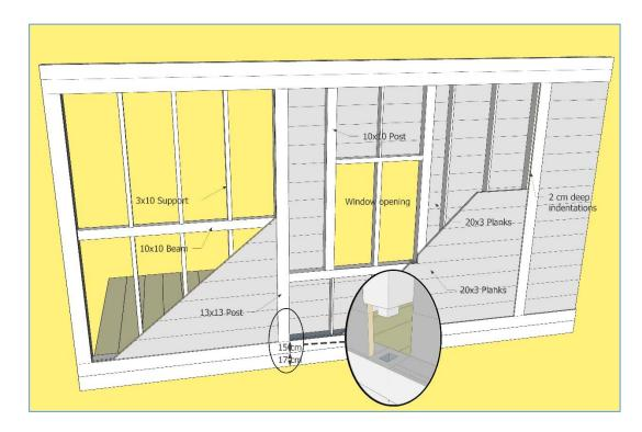
Figure 3.19. Construction detail of the timber infill technique.
