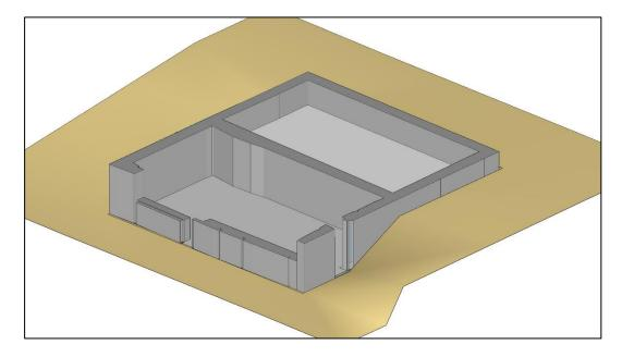
Figure 4.12. Masonry walls of the ground floor and foundation of Şenköy 3
