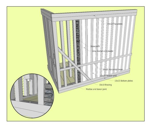
Figure 3.16. Construction detail of the çatma technique
