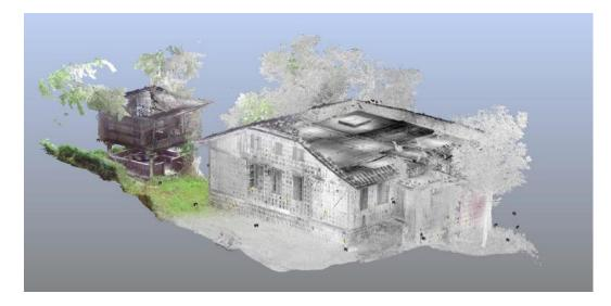
Figure 1.2. 3D point cloud of Şenköy 3
