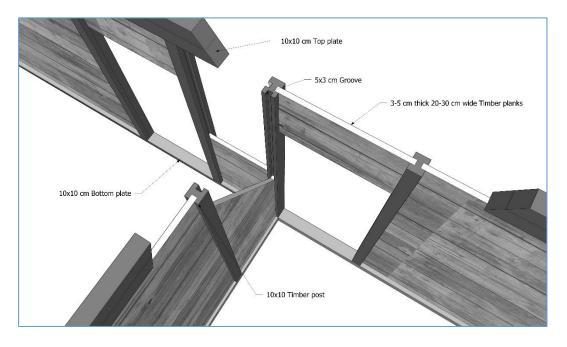
Figure 3.21. Construction detail of the taraba technique.
