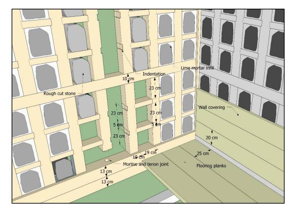
Figure 3.9. Construction model of the dolma göz technique
