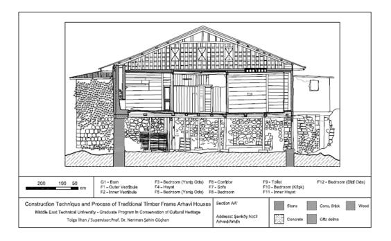
Figure 1.3. A section drawing of Şenköy 3 produced from the data taken from 3D point cloud With the newly gained information, another site survey was planned in 2016. 10 more houses were surveyed in seven days by measuring with laser distance meter and tape measure, drawing hand sketches, taking photographs. Access to the houses were difficult and the purpose was to study various cases in the villages of Arılı, Yolgeçen,
