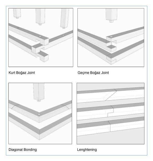
Figure 3.24. 3D representations of joint types seen in Arhavi
