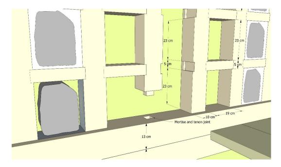
Figure 3.10. Construction detail of the dolma göz technique
