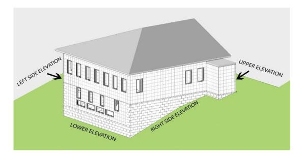
Figure 2.32. Alternative naming of the elevations that will be used in this study for clarity
