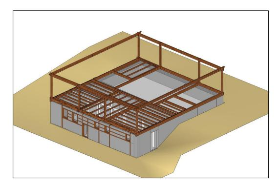
Figure 4.19. Placement of the floor joists
