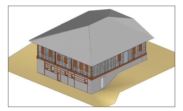
Figure 4.29. Placement of the corrugated metal sheet roof covering
