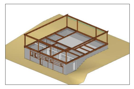
Figure 4.18. Post and beam system of the first floor
