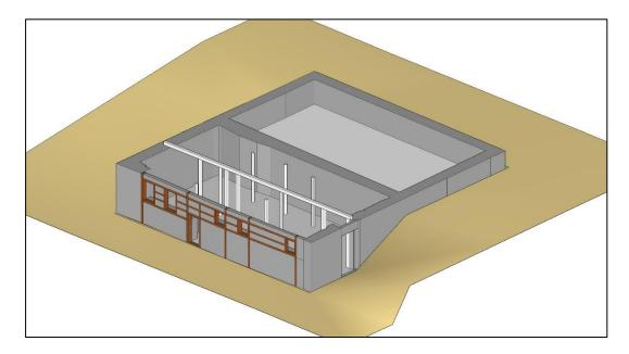
Figure 4.13. Timber frame lower wall of the ground floor of  $\S$ enköy 3
