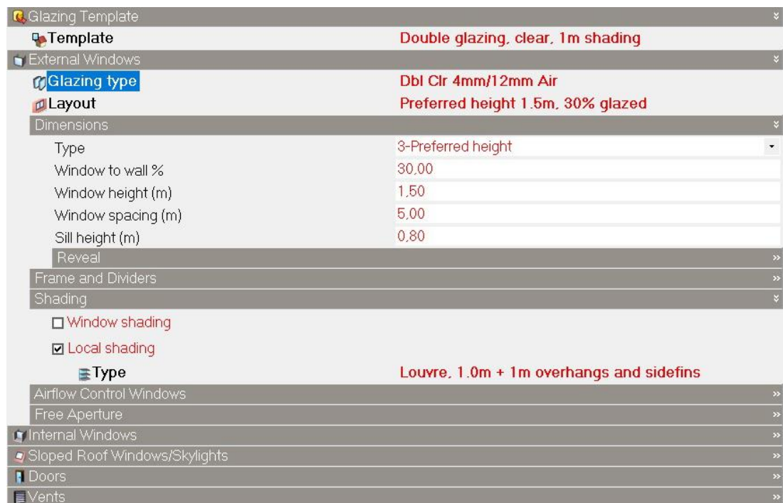
Figure A.7. Opening properties of the shadings for the renovation (R2.3.2)
