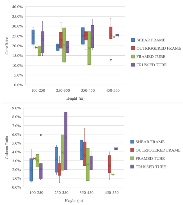
Figure 4.12. Core and column ratio distribution based on different height range in different structural systems in SG3
