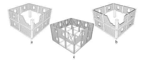
Figure 4.31. Sketches about common structural system and infill wall material in Turkey
