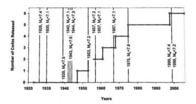
*Figure 1.1.* Demonstration of the relationship between the code development and the major earthquakes (Bal, 2007)
