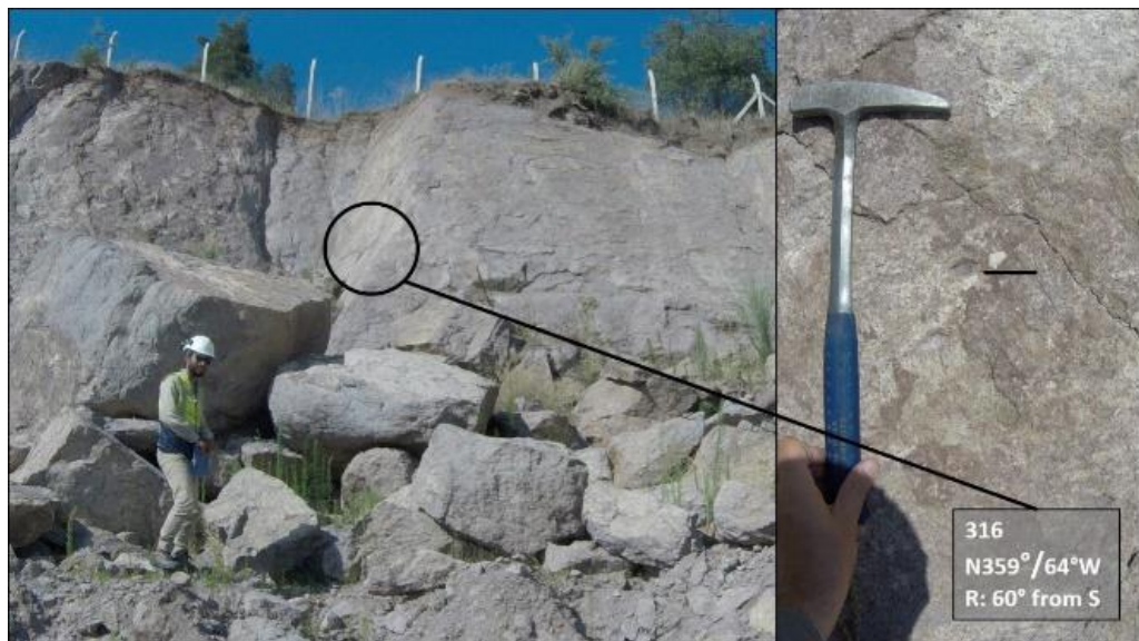
Figure 3.9. Field views from ca. N–S-trending normal fault with sinistral component; 1200 m east of Arzu South open pit with field ID 316; fault plane is 359°N/64°W, R= 60°S.
