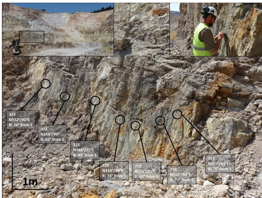
Figure 3.2. Field views from the Arzu South open pit 310 m level: Northwest–Southeast-trending pre- and/or syn-mineralizing normal fault with minor dextral component occurs at the contact of the main Arzu South low sulfidation Au-Ag quartz-adularia vein with field ID 317.
