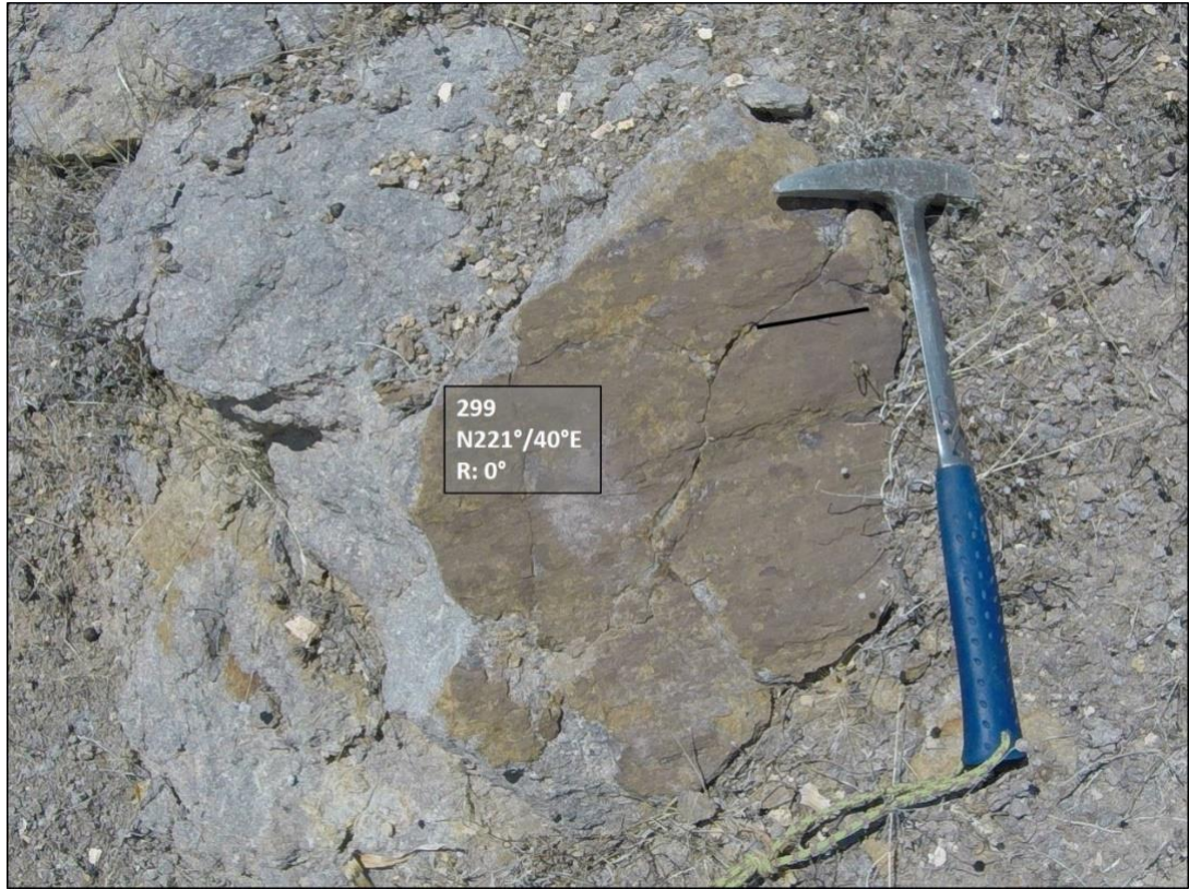
Figure 3.18. Field views from NE–SW-trending southeast-dipping syn-mineralizing dextral fault; north of Çaygören Dam with field ID 299; fault plane is 221°N/50°SE, R= 00°.
