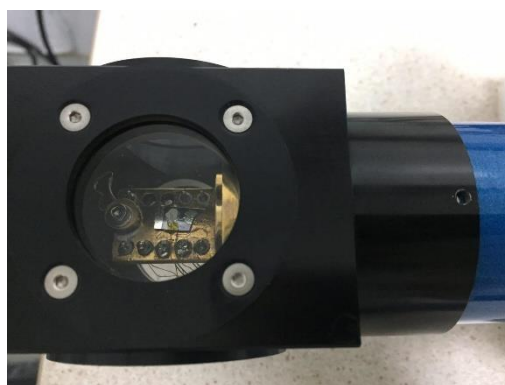
Figure 2.6. Shielded cryostat with sample placed on the electrode
