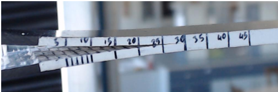
Figure C 3 Crack growth along the specimen under loading.
