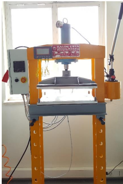
Figure 3.7 Hot press used for curing composite laminates.
