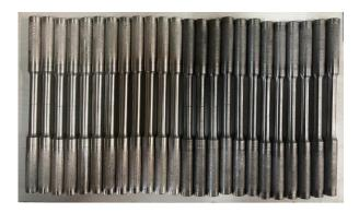
*Figure 4.5.* All the round specimens prepared for the test including the spares (12 on the left hand-side are Al and 12 on the righthand- side are steel)
