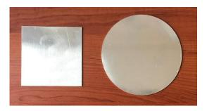
*Figure 4.25.* Specimen geometry for square cup test is on left-hand side. Specimen geometry for cylindrical and hemispherical specimens is on the right-hand side.
