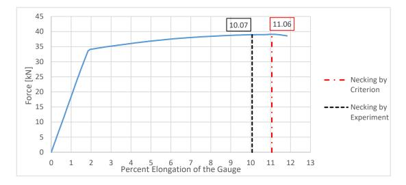
*Figure 6.24.* Punch force vs. percent gauge elongation of Element 100 for straight cross-section, round, Al specimen (Necking at 11.06% total elongation)
