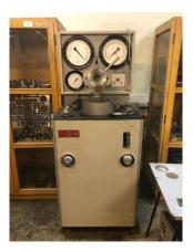
Figure 4.24. Tinius-Olsen Ductomatic A-40 Sheet Metal Tester
