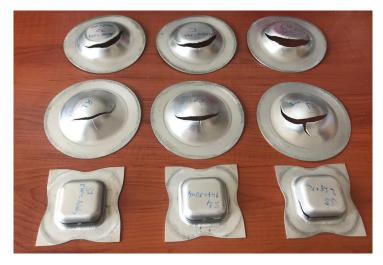
Figure 4.26. Deep drawing process specimens after completion of processes
