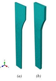
Figure 5.12. Mesh domain covering ¼ of the specimen (a) Al2024T3 (b) S235JR
