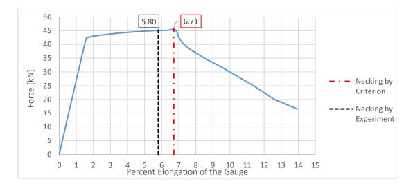
*Figure 6.60.* Punch force vs. percent gauge elongation of Element 100 for straight cross-section, round, steel specimen (Necking at 6.71% total elongation)
