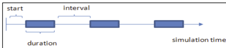
Figure 6.18. Failure settings of a resource in Tecnomatix Plant Simulation 14
