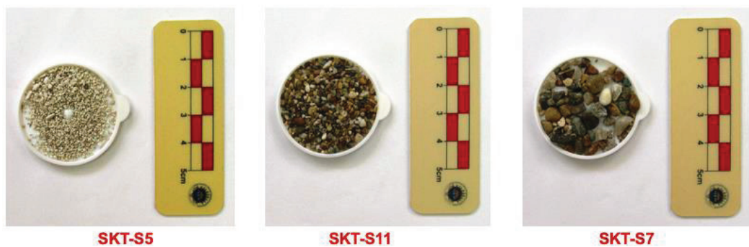
Figure 4.4. Aggregates after asidic treatment
