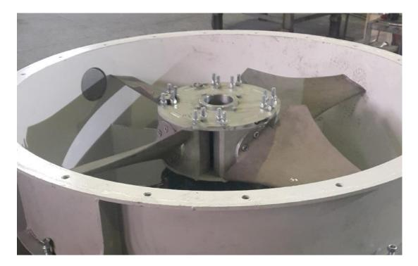
Figure 5.5. Assembled Impeller
