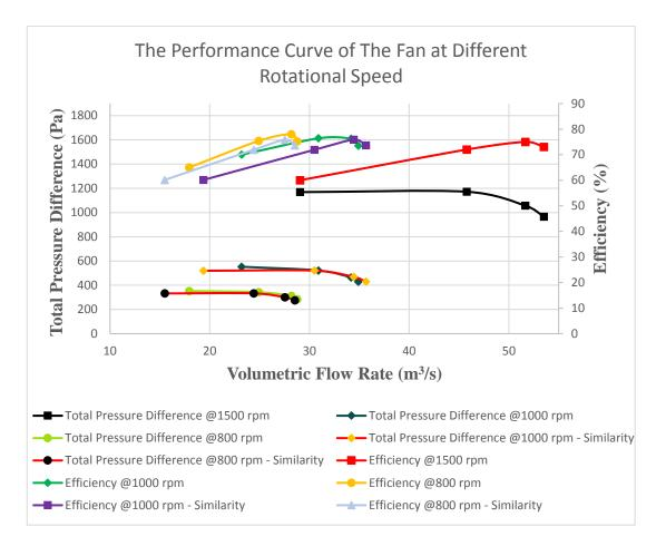
Figure 5.16. Comparison of Experimental and Similarity Performance Curves
