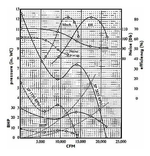
Figure 2.13. Performance Curves at 1750 and 2625 rpm [2]
