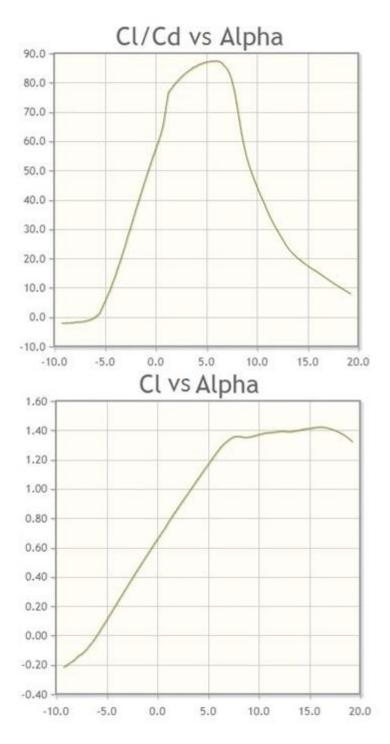
Figure 3.4. Lift and Drag Coefficients of NACA6409 [32]
