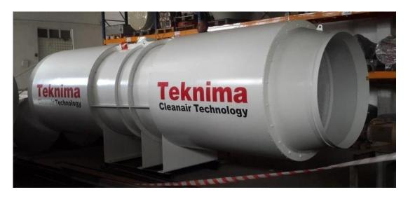
Figure 5.6. Assembled Axial Flow Fan
