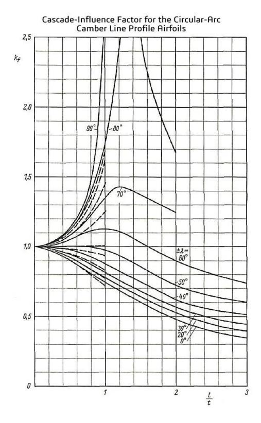
Figure 2.4. Cascade-Influence Factor for the Circular-Arc Camber Line Profile Airfoils [18]
