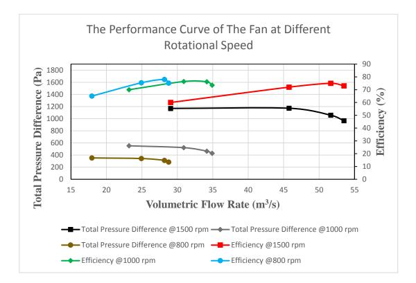
Figure 5.15. Performance Curves of the Fan for Different Rotational Speeds
