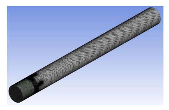
Figure 4.3. Meshed View of the Axial Fan Geometry
