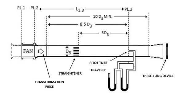
Figure 5.7. Outlet Duct Setup-Pitot Traverse in Outlet Duct [8]
