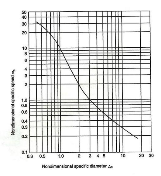
Figure 2.6. Cordier Diagram for Fans [16]
