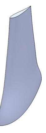
Figure 4.1. 3D Model of the Designed Fan Blade
