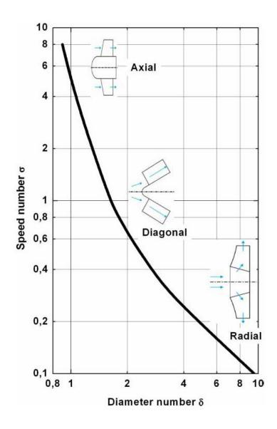
Figure 2.7. Classification of Impeller Types on the Cordier Diagram [20]
