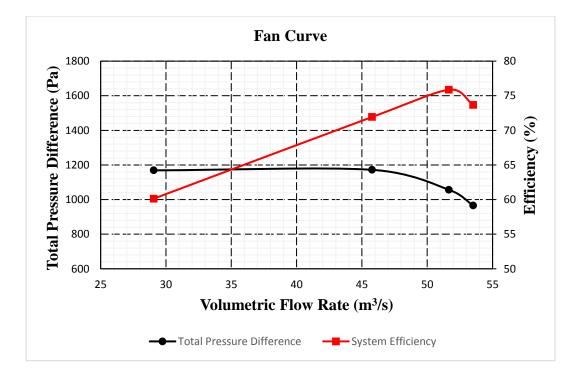
Figure 5.13. Experimental Performance Curves of the Axial Fan
