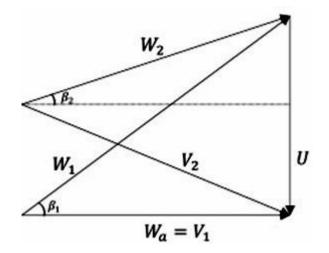
Figure 2.3. The Velocity Triangles Applied on an Airfoil
