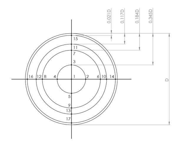
Figure 5.9. Positioning of the Pitot Tubes
