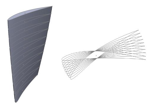
Figure 2.16. Sliced Fan Blade
