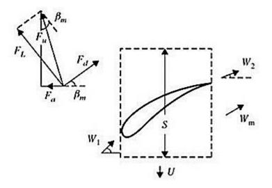
Figure 2.2. Forces Acting on Isolated Airfoil [16]
