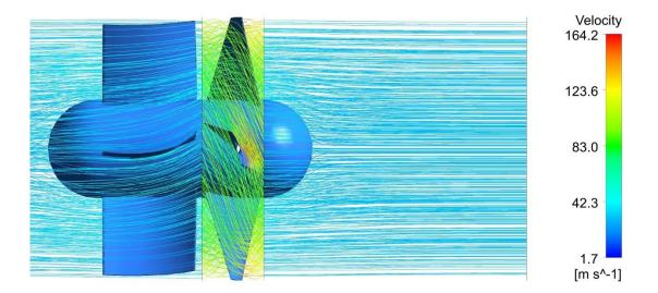
Figure 4.8 and Figure 4.9 shows the velocity streamlines in the fan.
