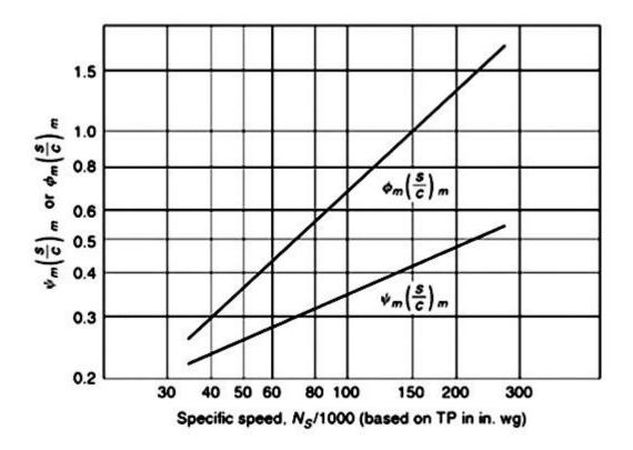
Figure 2.10. Specific Speed vs Flow and Head Coefficients [16]
