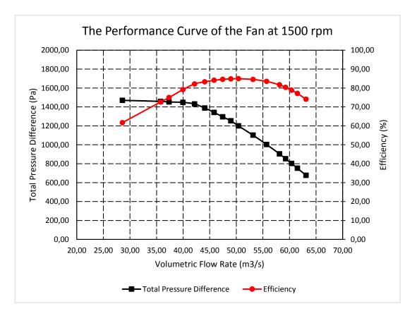
Figure 4.7. Calculated Performance Curves of the Fan
