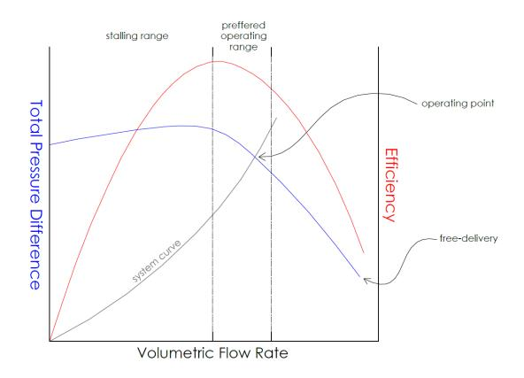
Figure 1.6. Performance Curves of an Axial Flow Fan
