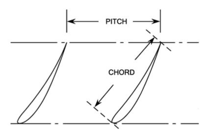
Figure 2.1. The Pitch Distance Between Fan Blades
