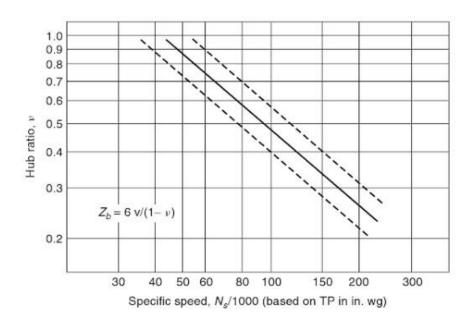
Figure 2.8. The Optimum Hub-Tip Ratio Range for Axial Flow Fans [16]
