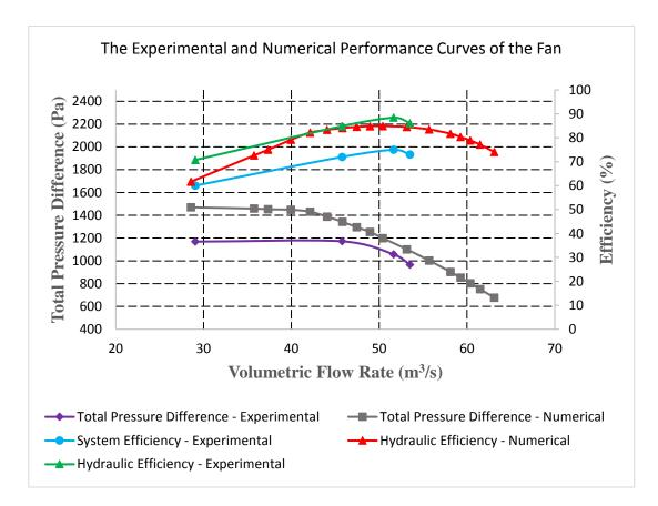
Figure 5.17. Comparison of Experimental and Numerical Performance Curves
