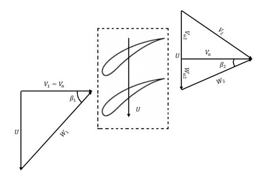
Figure 2.11. Velocity Triangles in Axial Flow Fan
