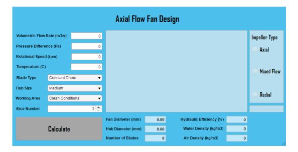
Figure 3.2. User Interface of Axial Flow Fan Design Software
