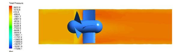
Figure 4.10. Total Pressure Distribution Throughout the Fan
