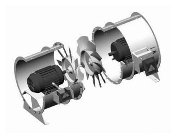
Figure 1.5. Two-Stage Axial Flow Fan without Guide Vanes [7]
