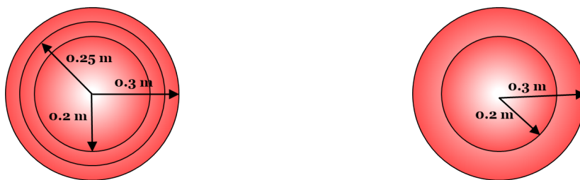
(a) Triple-layer modeling of a sphere with two inner spheres of radii 0.25 m and 0.2 m.
