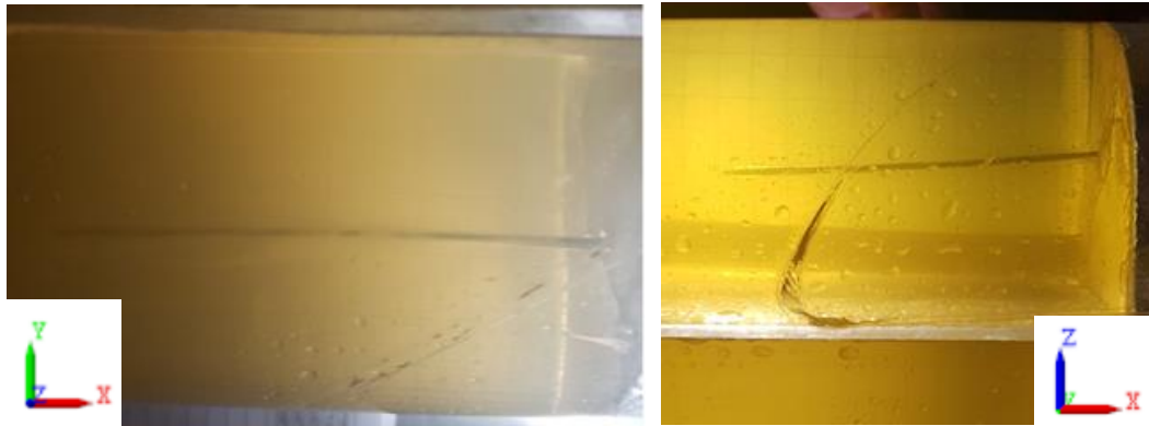
Figure 4.34. Deflection of needle in top and side view with 10mm needle advancement in ballistic gel
