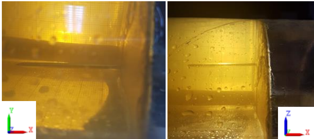
Figure 4.33. Deflection of needle from top and side view with 5mm needle advancement in ballistic gel
