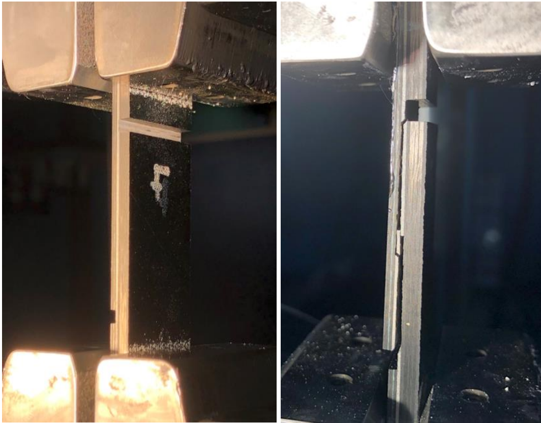
Figure 5.16. Uncracked and cracked specimen
