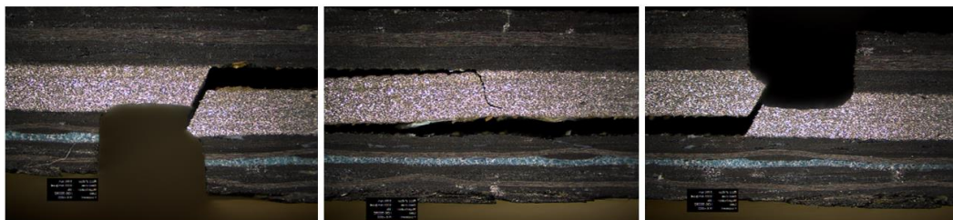
Figure 5.31. Microscopic examination of Specimen B5_T10_L40 SLJ
