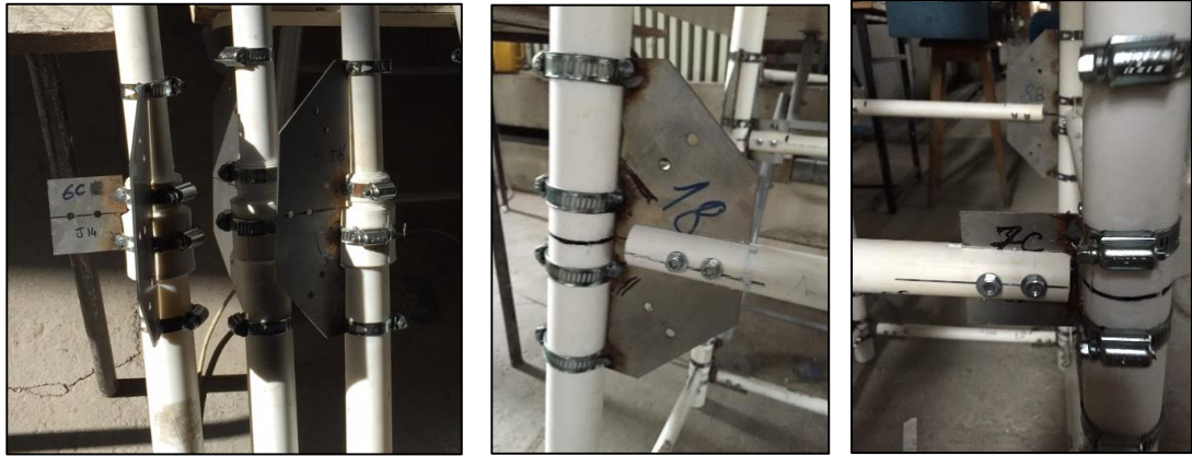
Figure 3.3. Joining of Connection Plates to the Members
