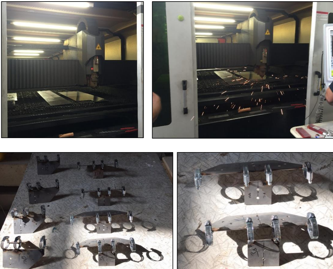
Figure 3.2. Ready to Use Connection Plates after Cutting and Welding
