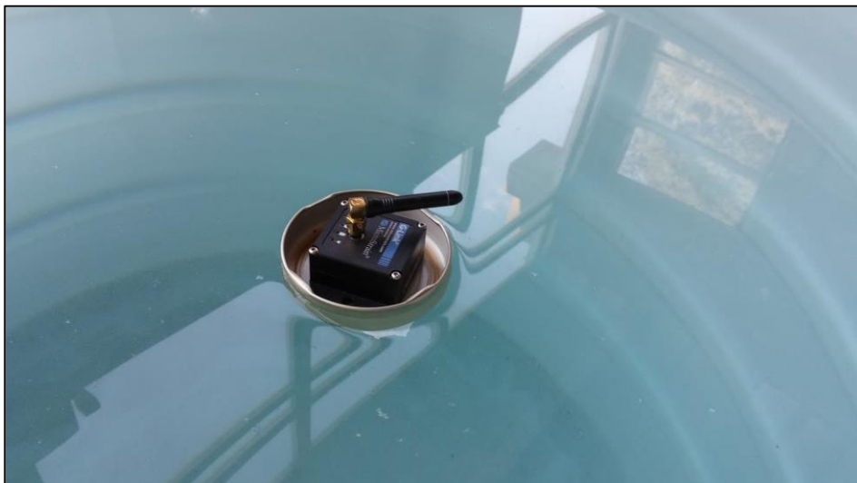
Figure 4.8. Prototype Measuring Device (Triaxial Accelerometer) Developed to Measure Wave Characteristics in the Pool
