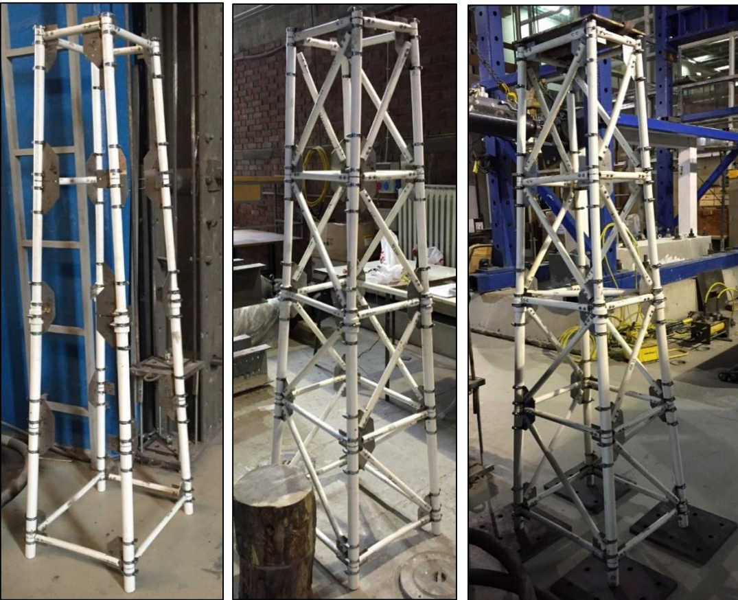
Figure 3.6. Stages of Physical Model Construction
