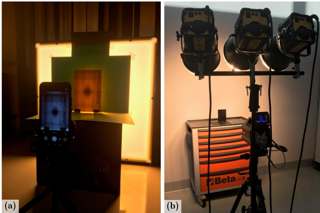
Figure 4.4. Post-mortem damage visualization of (a) GFRP specimens using a monochromatic light source, and (b) CFRP specimens using an optical infrared thermography setup.
