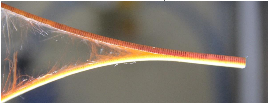
Figure 3.52. Side view of specimen #3 (G-DCB-ENF-45-45-7-MF10745) during DCB test
