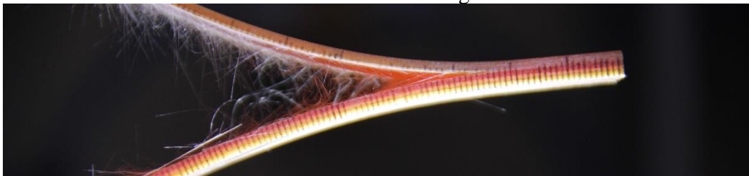
Figure 3.60. Side view of specimen #1 (G-DCB-ENF-90-90-11-MF10723) during DCB test
