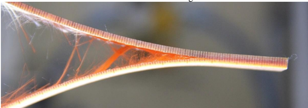
Figure 3.48. Side view of specimen #2 (G-DCB-ENF-45--45-10-MF11608) during DCB test
