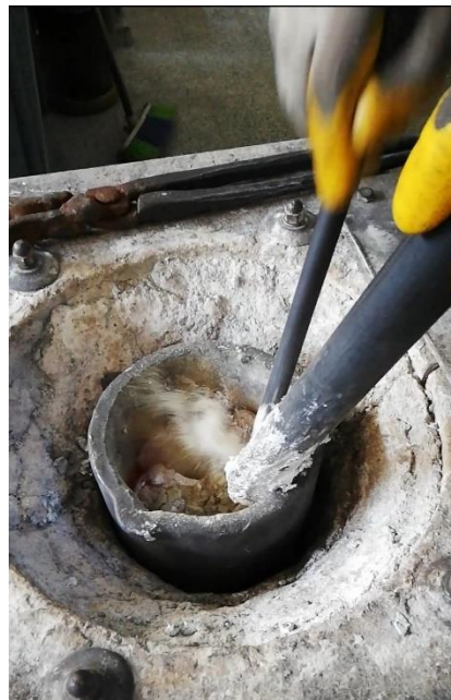
Figure 3.12. Melt stirring with graphite rods during alloy preparation
