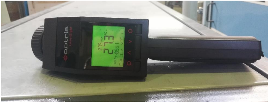
Figure 3.17. Optical pyrometer used to read die temperature
