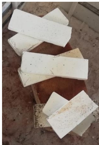
Figure 3.10. Sintered alumina preforms in resistance furnace
