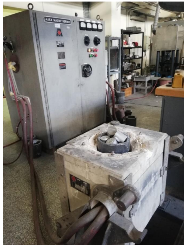
Figure 3.11. Induction melting furnace used for alloy preparation and melting
