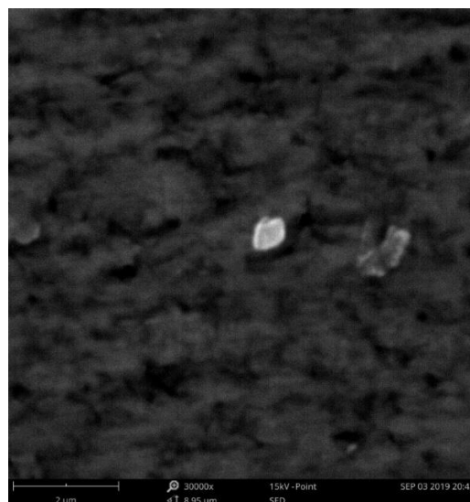
Figure 4.26. SEM image of precipitate that formed during aging step in T6 heat treatment
