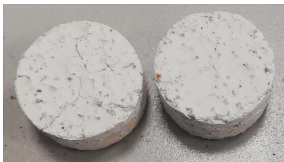
Figure 4.8. Crack formation in ceramic pellets having high metal additive content
