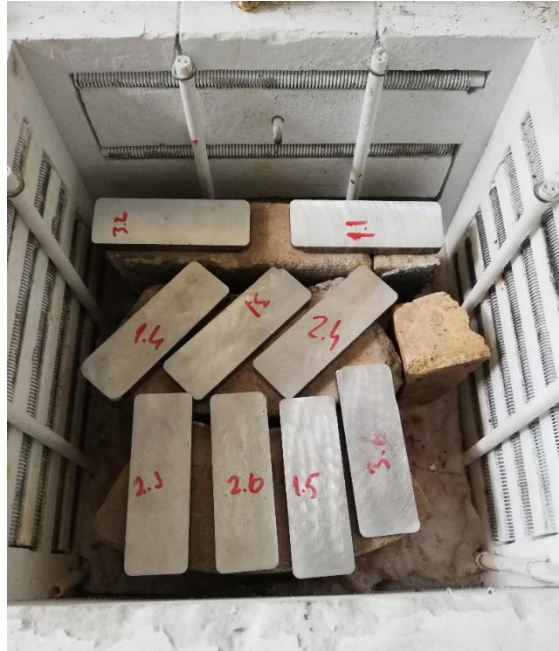
Figure 3.19. MMC samples in muffle furnace for solutionizing heat treatment
