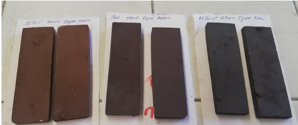
Figure 3.9. Sintered olivine preforms for pressure infiltration casting and three point bend testing
