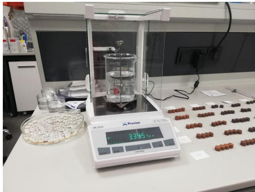
Figure 3.24. Archimedes density measurement
