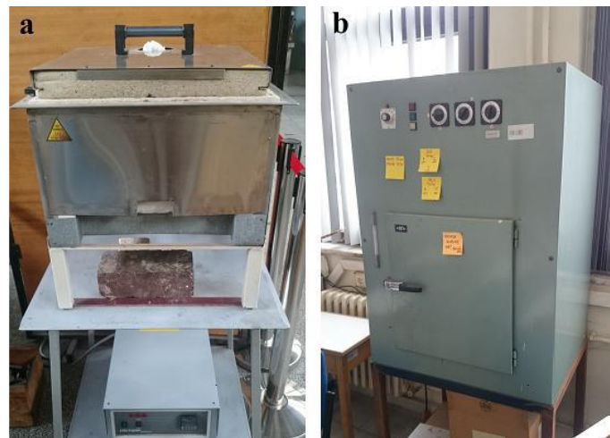
Figure 3.20. T6 heat treatment furnaces a.) Muffle b.) Electrical resistance furnaces
