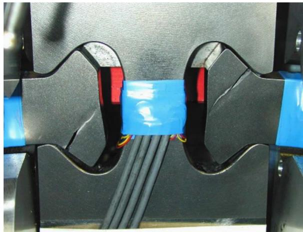
Figure 1.2. Failure in dovetail joint due to fretting [5]
