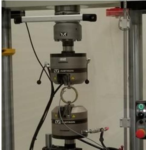
Figure 2.3. Proving ring calibration setup
