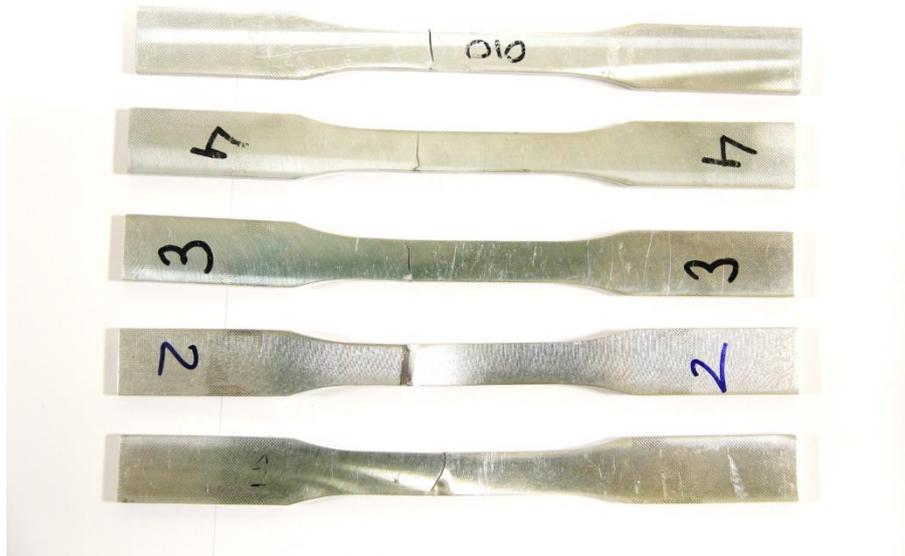
Figure 3.25. Specimens that have failed due to fretting fatigue (steel-aluminum contact)
