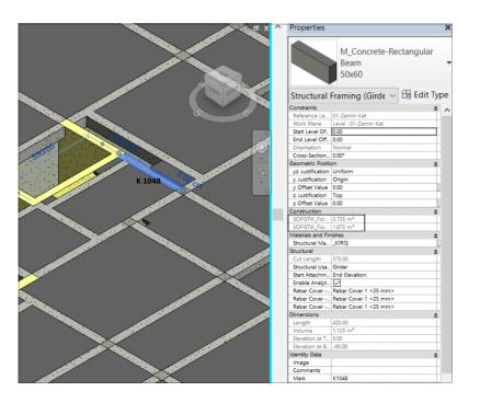
Figure 4.14. Beam Having Shaft Opening at One Side in Revit Model
