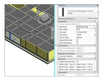
Figure 3.3. A Shorter Column due to Low Floor
