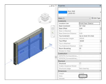
*Figure 3.12.* Area of an Architectural Wall (Exterior Face not Aligned with Structural Frame - after Using Join Feature of Revit)
