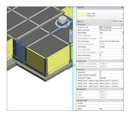
Figure 3.4. A Shorter Structural Wall due to Low Floor
