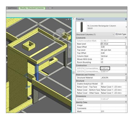
Figure 4.4. Incorrect Formwork Area of S11 Column in Revit Model
