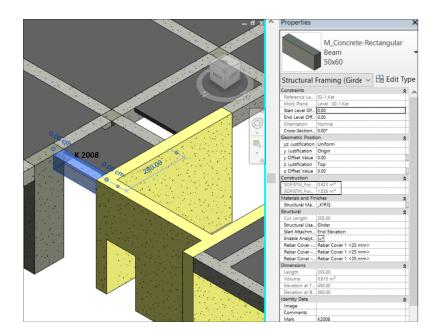
Figure 4.15. Beam Joining with Structural Wall in Revit Model
