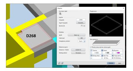
Figure 4.16. Incorrect Floor Thickness in D268 Floor in Allplan Model
