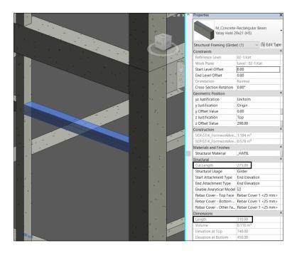
Figure 4.22. Beam having Unequal Length and Cut Length
