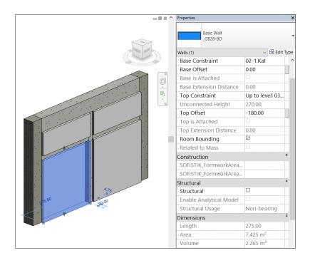
Figure 3.14. Architectural Wall with Coating
