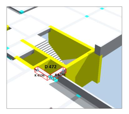
Figure 4.7. Missing Floor in Allplan Model
