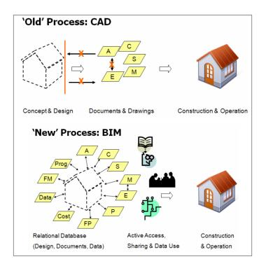
*Figure 2.3.* Comparison between Conventional CAD and New BIM Approach (Azhar et al., 2008)
