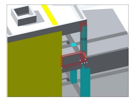
Figure 4.3. Modeling Mistake in Joint of Column and Parapet Wall in Allplan Model
