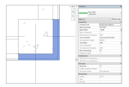
Figure 3.22. A Proper Joint of Insulation Elements in 2D Plan
