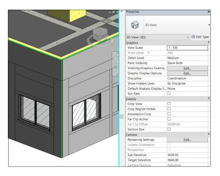
Figure 3.17. An Improper Joint of Insulation Elements in 3D Plan
