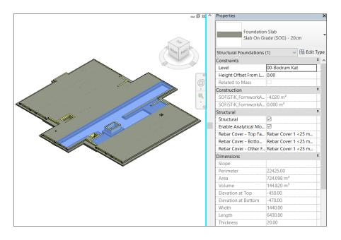
Figure 4.1. Foundation with Slab on Grade
