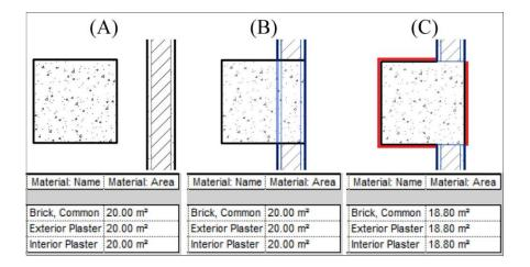
*Figure 2.4.* Comparison of Walls Quantity Take-off in Different Situations (Khosakitchalert et al., 2018)
