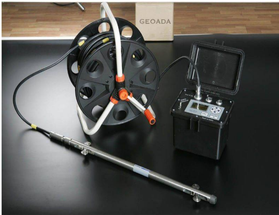
Figure 2.16. Typical Inclinometer System including Probe, Cable, Readout Unit (source: http://www.geodata.com/geodata-aletsel-gozlem-cihazlari.html ) [last accessed on 04.05.2019]
