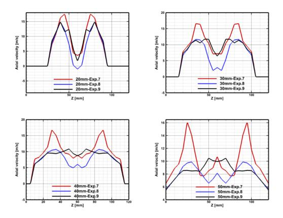
Figure A.7 Axial Velocities for Experiment 7,8 and 9
