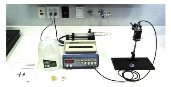
Figure 3.1 Droplet Generator System
