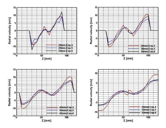
Figure A.2 Radial Velocities Experiments 4, 5 and 6
