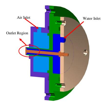
Figure 2.2 First Alternative Design for Inner Geometry
