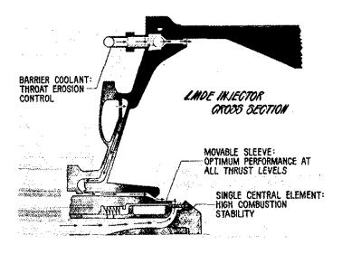
Figure 1.1 Lunar Module Descent Engine Pintle Injector [2]
