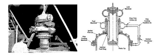
Figure 1.20 Technical Drawing and Injector Itself of LCPE [11]
