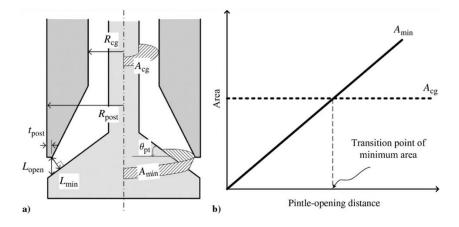
Figure 1.4 a) Base Geometry of the second work of Son et al [4] b) Pintle opening distance vs transition point [4]
