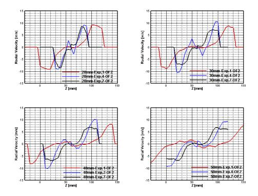
Figure 3.23 Radial Velocities for Experiment 1,4 and 7
