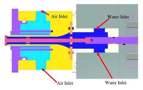
Figure 2.8. Cross Section of Moveable Mechanism from Top
