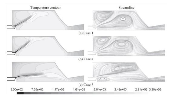
Figure 1.8 Comparison of Post Center Radius Effect From the Study of Son et al [7]
