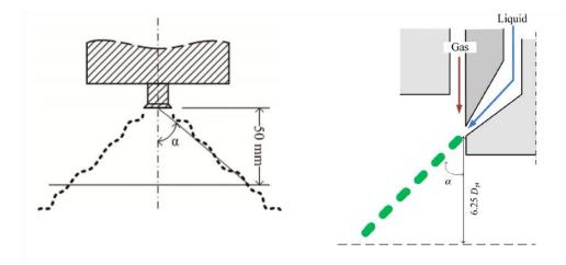
Figure 1.5 Cone Angle Defined by Son et al (on left [6], on right [5])
