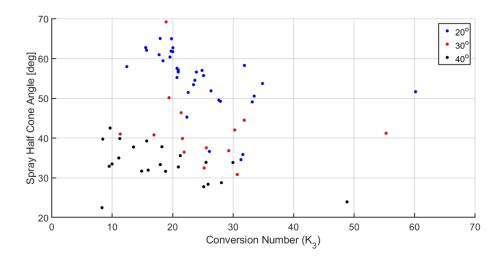
Figure 3.29 Characteristic Number vs Spray Half Cone Angle
