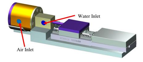
Figure 2.6 Movebale Mechanism with Linear Actuator
