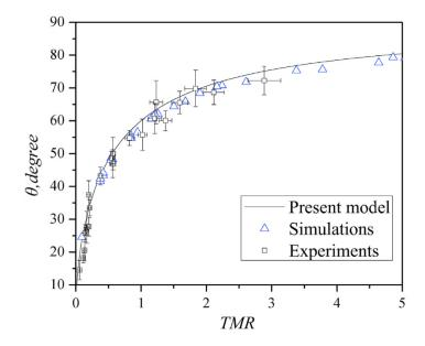
Figure 1.17 Comparison of 3 Ways to Determine Cone Angle
