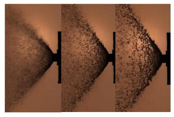
Figure 3.27 Spray Cone Formation of Experiment 10,11 and 12
