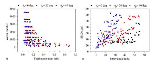
Figure 1.9. Weber Number-Total Momentum Ratio Relation for 3 Different Pintle Tip Angles [5]
