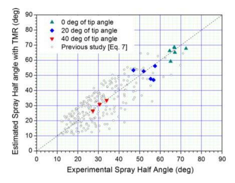
Figure 1.12 Comparison with atmospheric tests [15]
