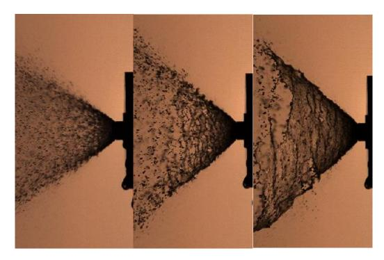
Figure 3.28 Spray Cone Formation of Experiment 4,5,6
