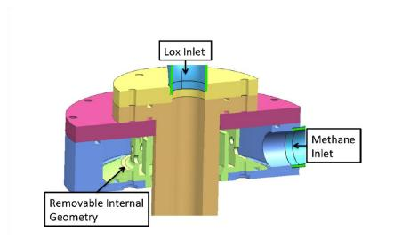
Figure 1.13. Base Geometry of Badard et al [8]
