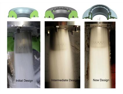
Figure 1.15. Uniformity of the Jet Intruduced by Bedard [8]
