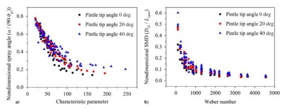
Figure 1.10 Spray Angle-Characteristic Number Relation for 3 Different Pintle Tip Angles [5]
