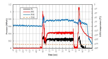
Figure 1.19 Fuel-Centered Pintle Injector Hot Fire Test Done by Sakaki (Chamber Pressure, PFI: Fuel injection pressure, POI: Oxidizer injection pressure, TOI: Oxidizer injection temperature) [10]
