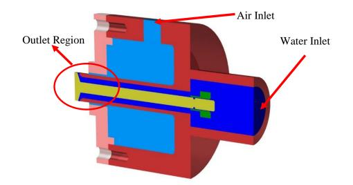
Figure 2.4. Second Alternative Design (Direct Flow Passage)
