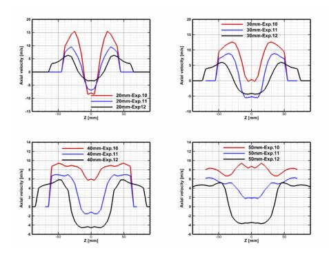
Figure 3.18 Axial Velocity Plots for Experiment 10,11 and 12
