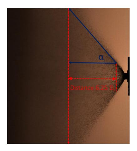
Figure 3.25 Spray Cone Angle Measurement with Shadowgraph Technique
