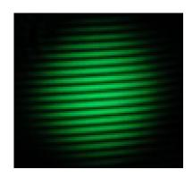
Figure 3.6 Sequential Pattern of Dark and Light Fringes at Crossing Volume
