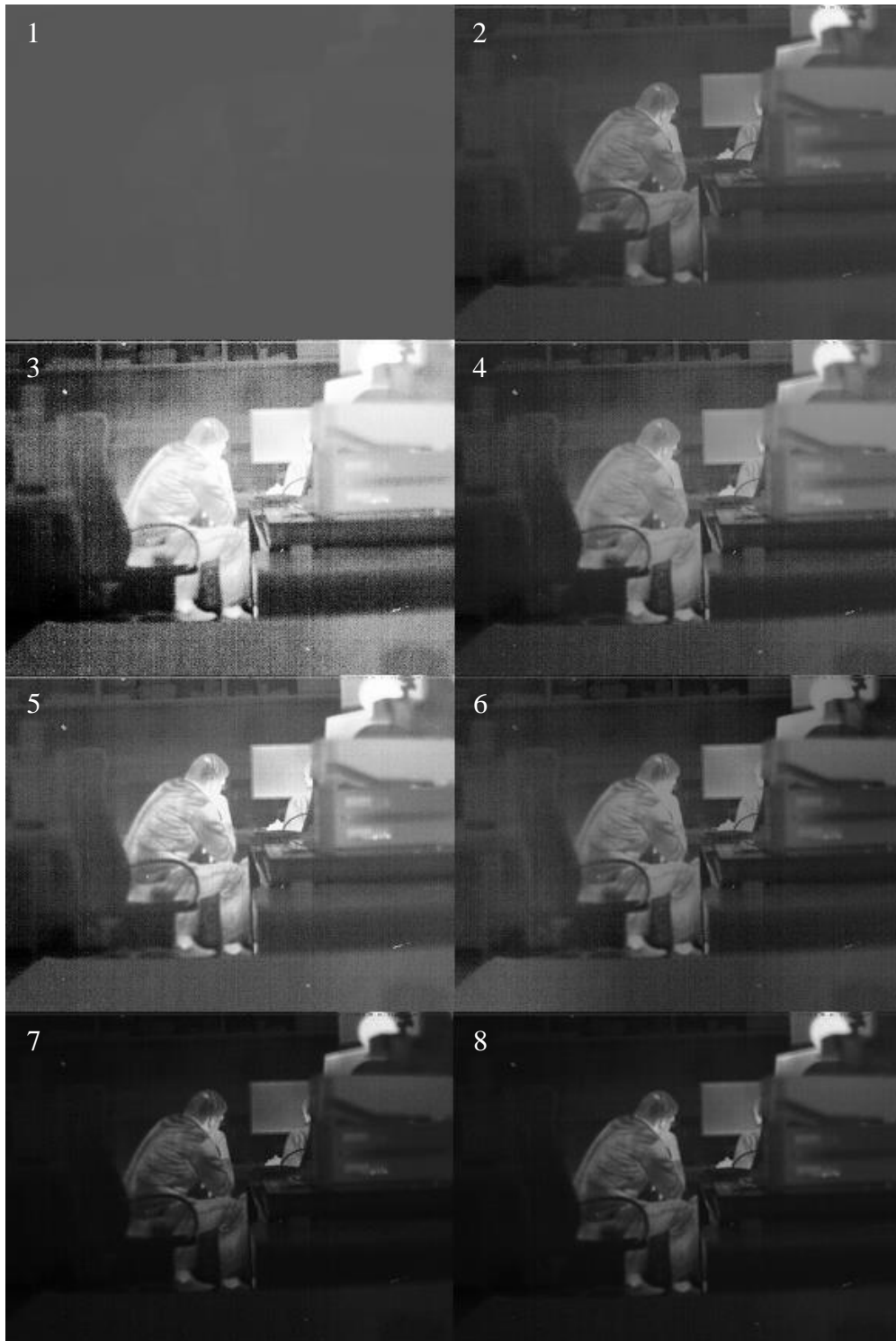
Figure 4.3. Comparison of 1) Raw image, 2) Contrast stretching, 3) Linear HE, 4) WMSHE, 5) ADPHE, 6) CLAHE, 7) MATLAB and 8) FPGA implementation of the proposed method
