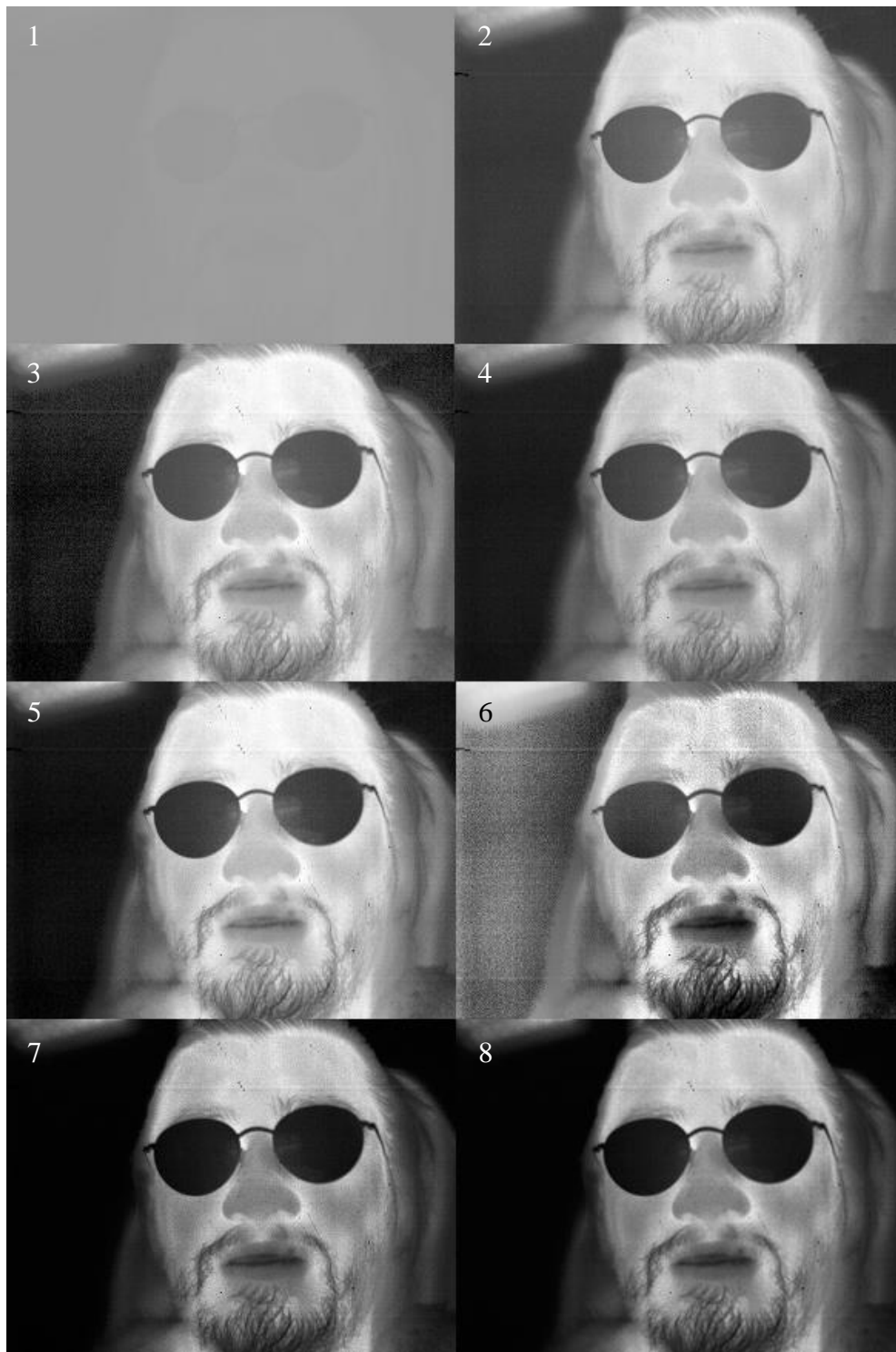
Figure 4.5. Comparison of 1) Raw image, 2) Contrast stretching, 3) Linear HE, 4) WMSHE, 5) ADPHE, 6) CLAHE, 7) MATLAB and 8) FPGA implementation of the proposed method
