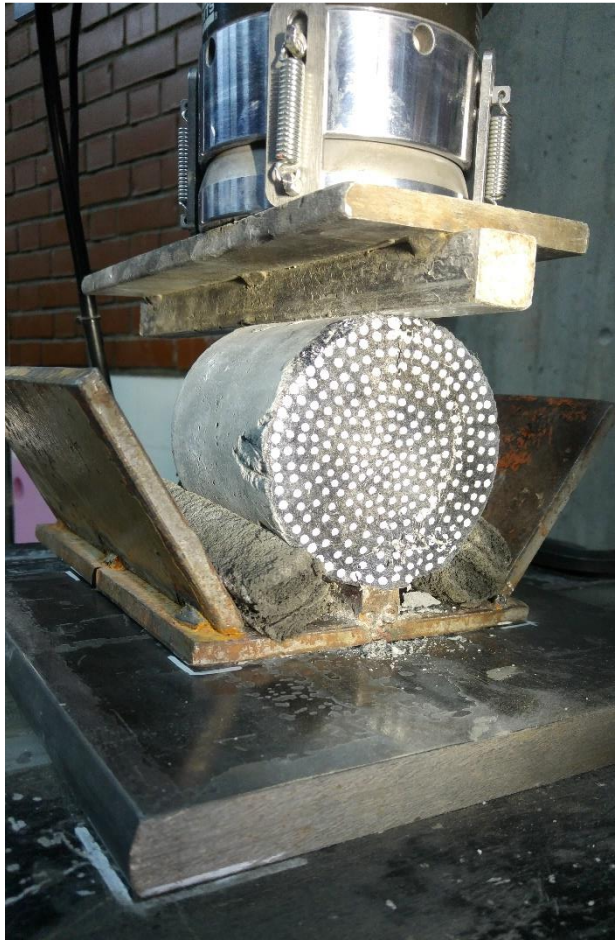
Figure 3.6. Splitting Tensile Strength Test
