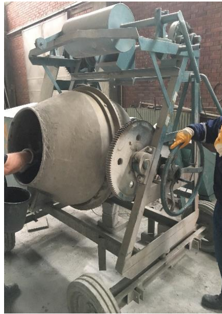
Figure 3.3. Rotary Drum Concrete Mixer
