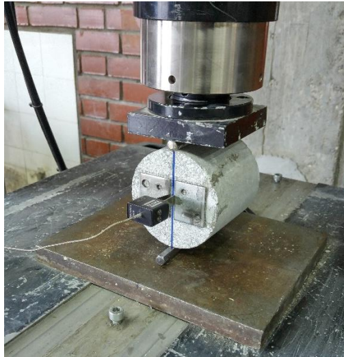
Figure 2.9. Splitting Tensile Strength Test Setup
