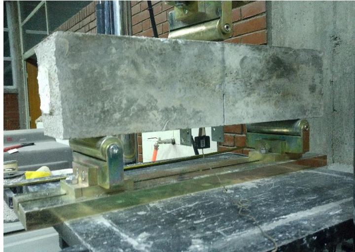
Figure 2.10. Single Point Loading, CMOD Test Setup
