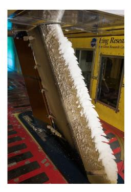
Figure 1.3. Ice accretion on a wing in an icing wind tunnel [18]
