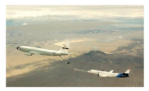
Figure 1.2. Icing tests in simulated clouds produced by icing tanker [9]
