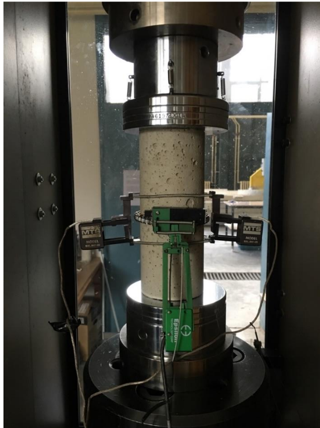
Figure 4.3. Static Deformability Test Setup
