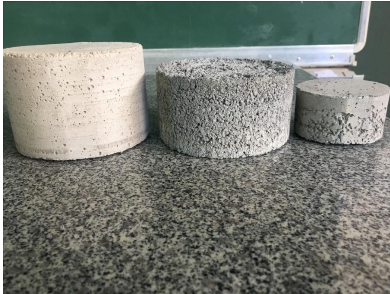
Figure 3.10. Successful and unsuccessful casting products
