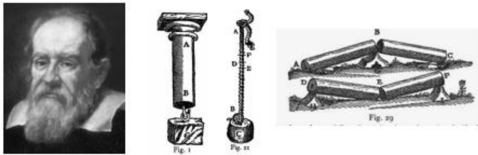
Figure 2.2. Galileo Galilei tensile test setup (Gross, 2014)
