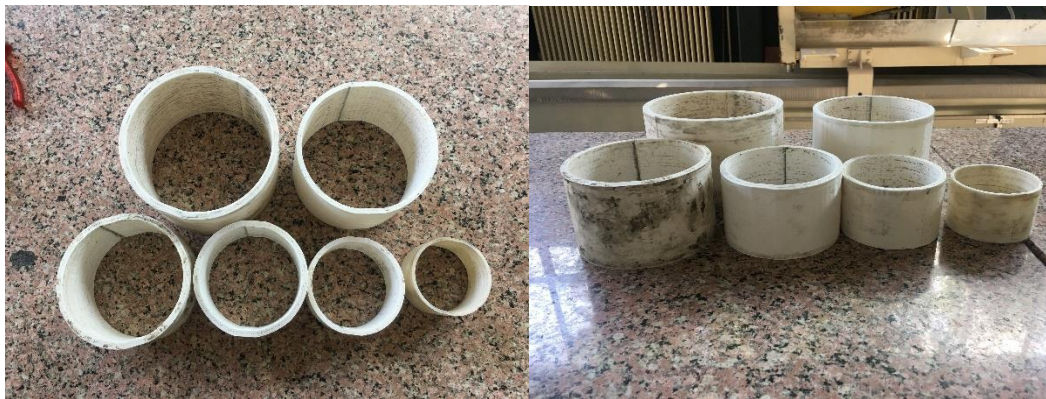
Figure 3.6. Used molds with varying diameters 100 mm to 200 mm
