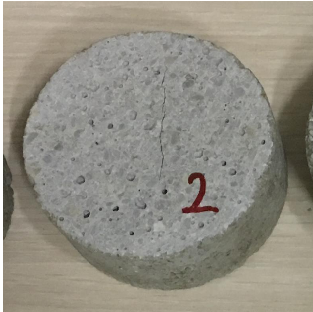
Figure 4.10. A typical Brazilian Disc sample with central crack clearly visible
