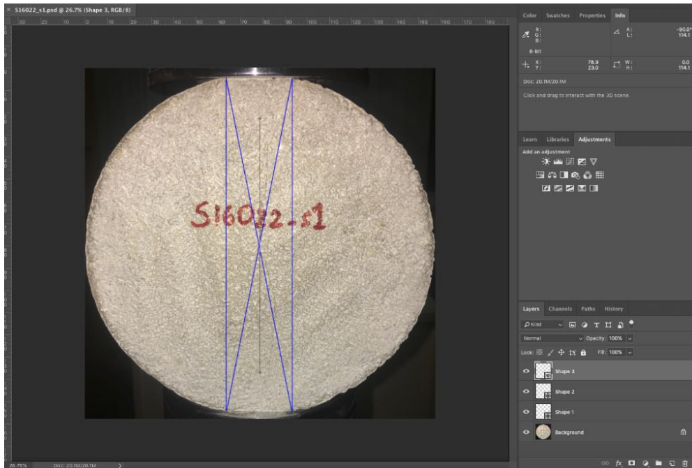
Figure 0.77. FBD test crack measurement of the sample S160_s1
