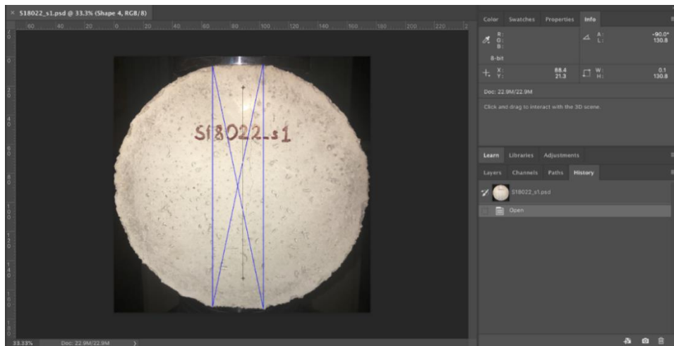
Figure 0.82. FBD test crack measurement of the sample S180_s1
