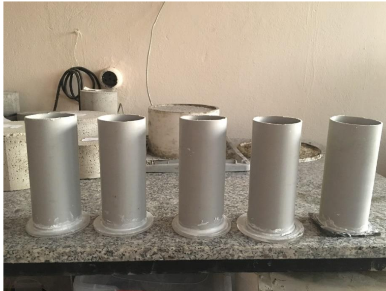
Figure 4.1. Prepared molds for conventional testing
