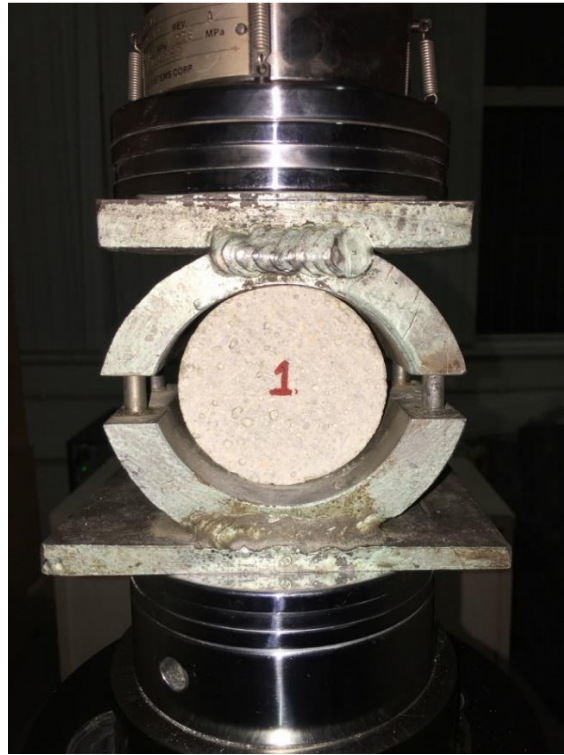
Figure 4.9. Brazilian Disc Test set up
