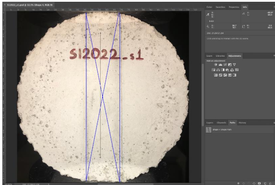
Figure 0.66. FBD test crack measurement of the sample S120_s1
