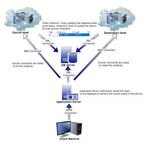
Figure 4.5: Clock Application Execution Plan
