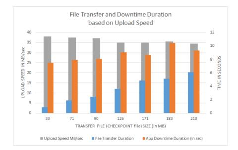
Figure 5.9: Upload Speed Effect on Downtime and File Transfer Duration
