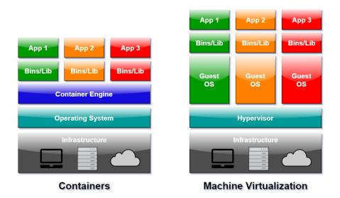
Figure 2.1: Containers versus Virtual Machines
