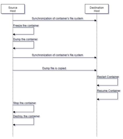
Figure 4.4: CRIU Principle Diagram [3]
