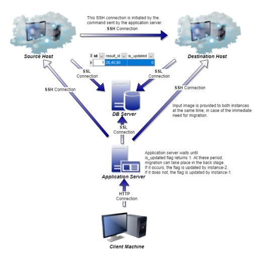
Figure 4.6: Face Recognition Application Execution Plan
