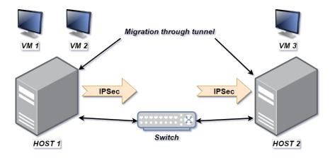
Figure 3.4: IPSec Tunneling [4]
