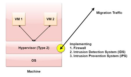
Figure 3.2: Network Security Engine Hypervisor [4]
