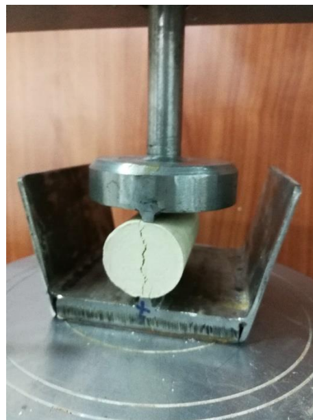
Figure 3-14. Specimen placement in direct tensile test
