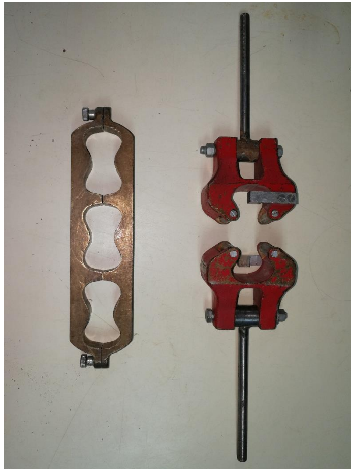
Figure 3-11. Special 8-shaped mold and direct tensile test apparatus
