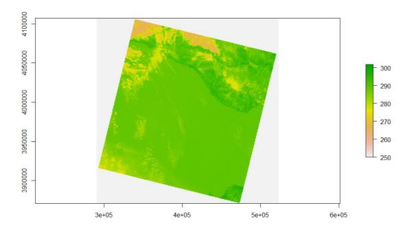
*Figure 2.24* Brightness Temperature (Kelvin) Result of LS8 Image LC08\_L1TP\_177035\_20180402\_20180416\_01\_T1 (Axes Represent UTM Coordinates)
