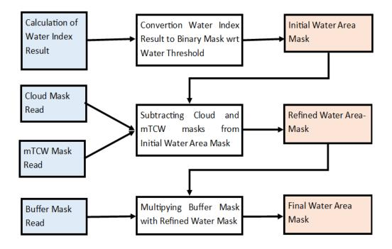
Figure 2.3 Flow Chart of the Model up to the Calculation of Final Water Area Mask
