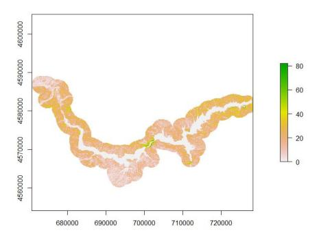
Figure 2.10 Slope Map (in Degrees) of Altınkaya Dam Buffer Area Based on ASTER DEM (Axes represent UTM coordinates)
