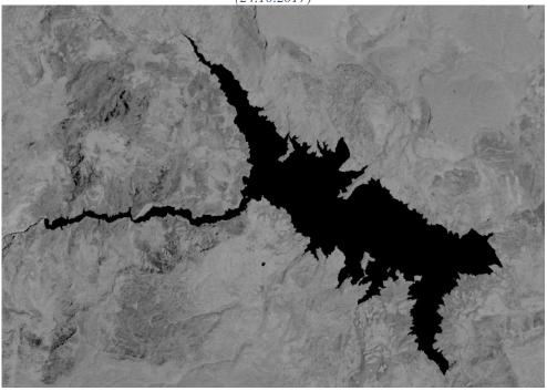
Figure 3.8 Water Area Detection based on NDPI Index over Ermenek Dam, Before Masking (15.07.2017)
