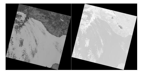
Figure 2.27 Whiteness Mask (Left) and Land Variance Mask (Right) calculations of the Cloud Mask of LS8 Image LC08\_L1TP\_177035\_20180402\_20180416\_01\_T1
