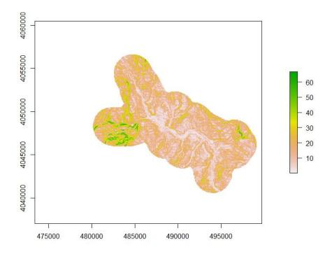
Figure 2.7 Slope Map (in Degrees) of Ermenek Dam Buffer Area Based on ASTER DEM (Axes represent UTM coordinates)
