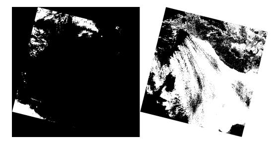
Figure 2.22 PCP (Left) and Water Mask (Right) results of LS8 Image LC08\_L1TP\_177035\_20180402\_20180416\_01\_T1
