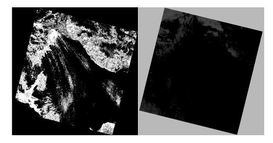
Figure 2.26 Clear Sky Land Mask (Left) and Temperature Based Cloud Probability Mask (Right) of LS8 Image LC08\_L1TP\_177035\_20180402\_20180416\_01\_T1
