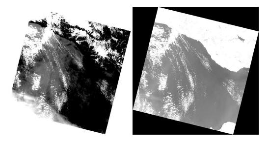
*Figure 2.25* Temperature Based Water Probability Mask (Left) and Brightness based Probability Mask (Right) of LS8 Image LC08\_L1TP\_177035\_20180402\_20180416\_01\_T1
