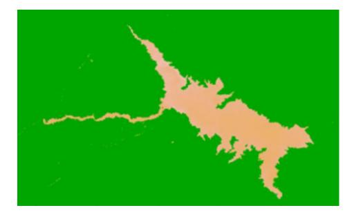
Figure 3.1 Detected Water Area of Ermenek Dam for 18/08/2016 (Green areas are land pixels)
