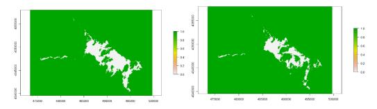
Figure 2.35 Result Plots of Ermenek Dam Area based on Different NDWI.MCF Thresholds (0.16 on the Left and 0.18 on the Right)
