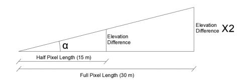
Figure 2.1 Demonstration of Elevation Change Within a Pixel and Half Pixel with respect to Slope
