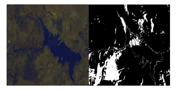
Figure 2.21 RGB Image (Left) and Related Cloud Mask Result (Right) of the LS8 Image LC08\_L1TP\_177035\_20160802\_20170322\_01\_T1
