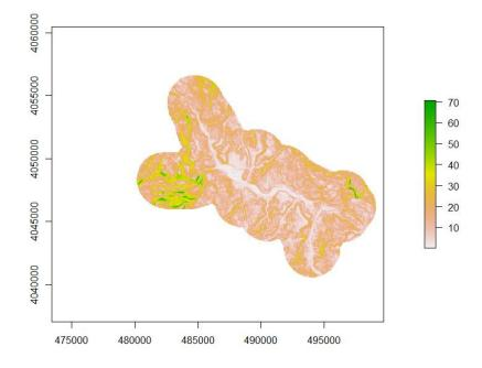
Figure 2.6 Slope Map (in Degrees) of Ermenek Dam Buffer Area Based on SRTM DEM
