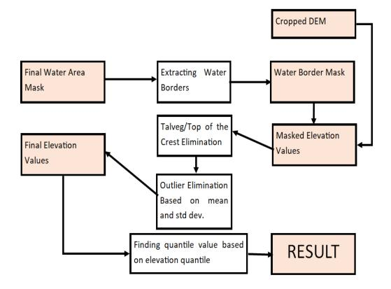
Figure 2.4 Flow Chart of the Model about Water Elevation Detection
