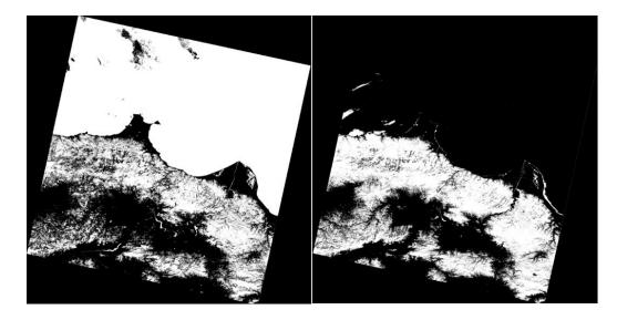
Figure 2.30 Results of AWEI-S (Left) and mTCW (Right) Calculations of Landsat-8 Image LC08\_L1TP\_173033\_20180201\_20180220\_01\_T1
