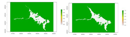
Figure 2.36 Result Plots of Ermenek Dam Area based on Different NDWI.MCF Thresholds (0.10 on the Left and 0.05 on the Right)
