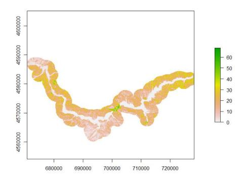
*Figure 2.9* Slope Map (in Degrees) of Altınkaya Dam Buffer Area Based on SRTM DEM (Axes represent UTM coordinates)
