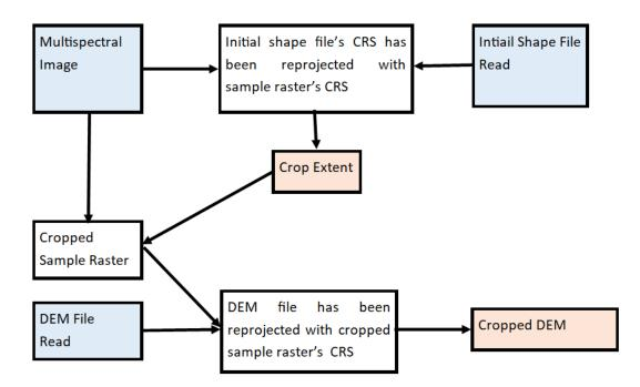
Figure 2.2 Flow Chart of the Model up to the Calculation of Cropped DEM
