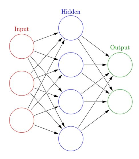
Figure 2.9: Artificial neural network figure is taken from [20]. Since binary classification is applied in this study, two nodes are used at the output layer to illustrate ANN.
