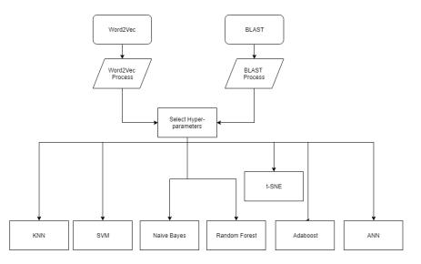
Figure 2.3: Flowchart of the proposed methods where the Word2vec model is trained with subsequences and feature vectors of these subsequences are fetched from the Word2vec model to compute feature vectors of protein sequences. With these feature vectors, classifiers are trained to predict Enzyme Commission classes.
