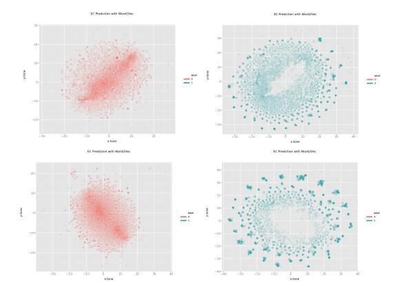
Figure 4.15: Vector representations of Word2vec models are visualized by using the t-SNE algorithm to project vectors onto 2D space. The first figure of second class belongs to the vector representations of the negative data items in the second class and the second figure of second class belongs to the vector representations of the positive data items in the second class. In order to compare the classes, vector representations of the fourth class are given at the second row of figures.
