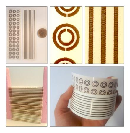
Figure 3.56: Photographs of a fabricated composite metamaterial. The design is shown in Figure 3.37.
