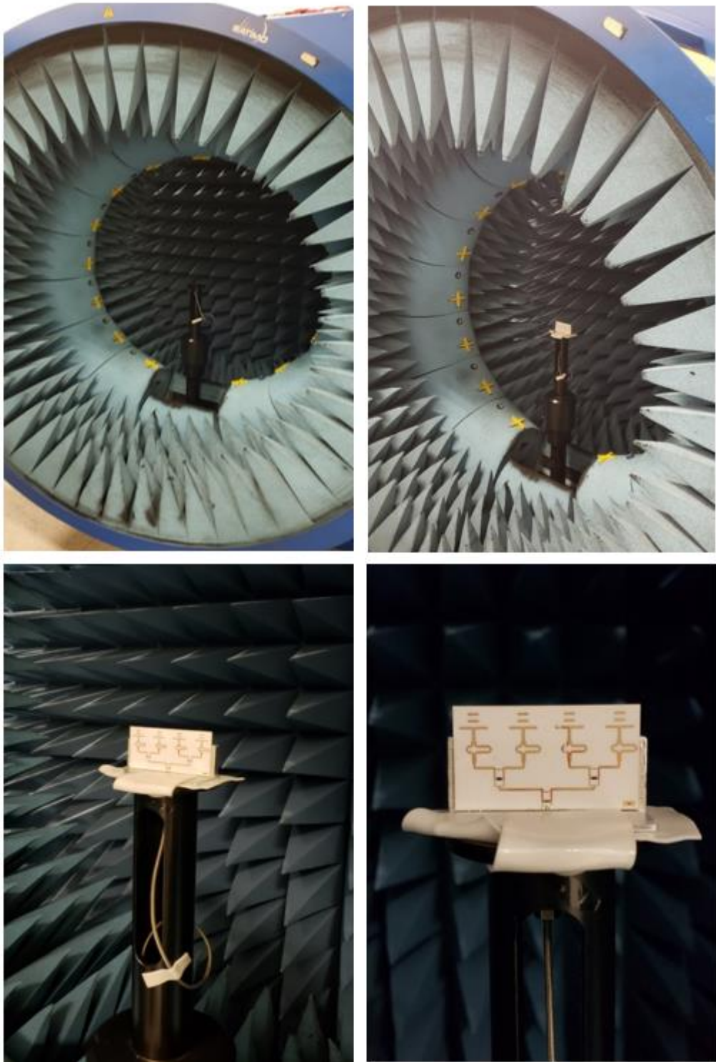
Figure 5.5. Four elements linear array antenna measurement setup
