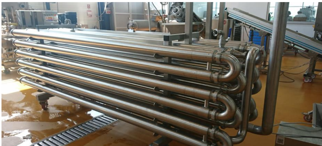
Figure 2.2. Tubular heat exchanger
