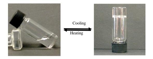
Figure 1.3. Heating and cooling cycle of thermo reversible supramolecular gels (Schön, 2014)
