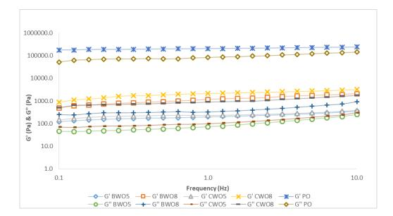
Figure 3.11. Storage and Loss Modulus of the Palm Oil & Oleogels
