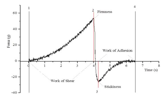
Figure 1.8. Measurement Curve of the Texture Profile
