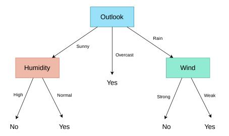
Figure 4.1: A decision tree example. Nodes are features, connections are values for each feature, and leaves are classes.
