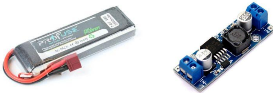
Figure 4.2. ProFuse 7.4 V Li-Po Battery and 5V 3A Voltage Regulator Card
